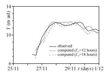
Figure 4.14: Comparison between observed and forecasted water levels with different lead times from the ANN model for the November 2005 flood. Source: Napolitano et al. (2009).
