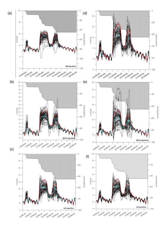
Figure 5.9: Results for a) Expts #23; b) Expt #24; c) Expt #25; d) Expt #26; e) Expt #27; f) Expt #28 for the 2008 flood event. The red line is the observed and the blue line is the average of the predictions. Cumulative rainfall is plotted on the top of each graph.
