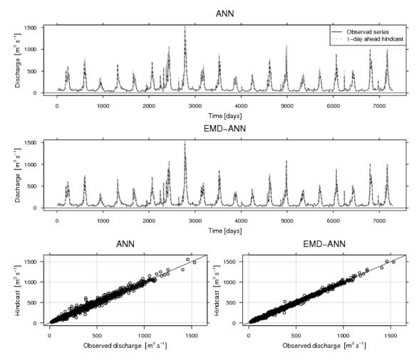
Figure 6.8: The Clark Fork River discharge time series of the test period along with 1-day ahead hindcasts obtained by (a) a simple ANN and (b) the EMD–ANN model. Scatterplots of the observed discharge vs hindcasts computed by (c) the ANN and (d) the EMD–ANN. Source: Napolitano et al. (2011).
