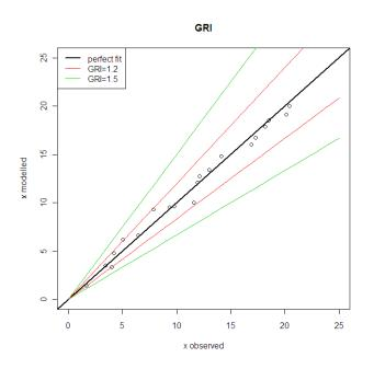
Figure 3.1: Visualisation of the GRI cones around the best fit line
