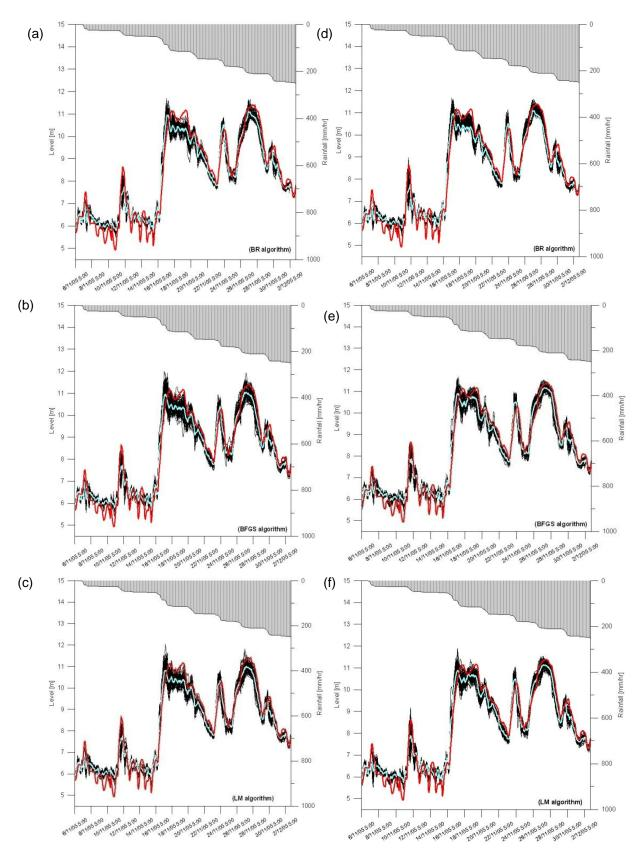
Figure 5.8: Results for a) Expts #17; b) Expt #18; c) Expt #19; d) Expt #20; e) Expt #21; and f) Expt #22 for the 2005 flood event. The red line is the observed and the blue line is the average of the predictions, shown individually in black. Cumulative rainfall is plotted on the top of each graph.
