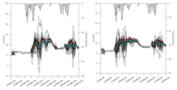
Figure 5.4: Results for a) Expt #6 and b) Expt #7 for the 2008 flood event. The red line is the observed and the blue is the mean of the 50 simulations, which are shown individually in black. Observed hourly rainfall is shown in grey at the top of both figures.
