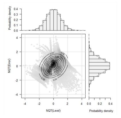
Figure 5.14 NQT applied to Expt #18. The figure shows the empirical joint histogram and the isolines of the joint Gaussian density function with a correlation parameter equal to the empirical correlation computed on the data. At the top and right are the histograms of the NQT variables and the corresponding standard Gaussian density functions (dashed lines).
