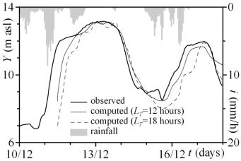
Figure 4.16: Comparison between the observed and forecasted water levels with different lead times for the TFF model for the December 2008 flood. Source: Napolitano et al. (2009).
