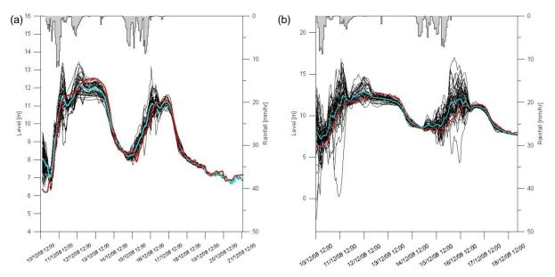
Figure 5.2: The 2008 flood event computed with (a) hourly rainfall (Expt #2) and (b) effective rainfall (Expt #3), where the red line is the observed and the blue is the mean of the 50 individual simulations, which are shown in black. Observed rainfall is shown in grey at the top of (a) and effective rainfall is shown at the top of (b).
