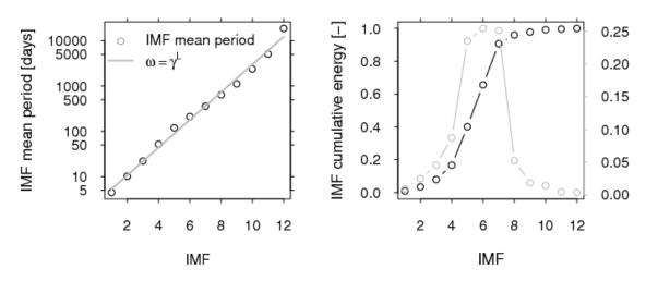
Figure 6.7: On the left is the scaling relationship between the number of IMFs and the corresponding mean periods for the components of the Clark Fork River time series. On the right is the non-dimensional energy (gray) and cumulative energy (black) for each IMF. Source: Napolitano et al. (2011).
