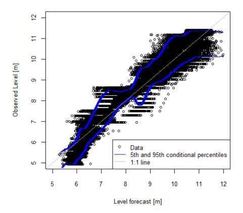
Figure 5.16: Quantile Regression with a spline of 25 degrees of freedom for Expt #18 for the observed versus forecast water levels
