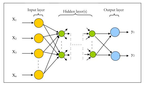
Figure 2.2: Schematic of a multi-layer ANN
