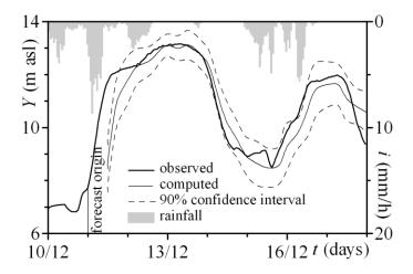
Figure 4.15: Comparison between the observed and 12h forecasted water levels for the TFF model for the December 2008 flood. Source: Napolitano et al. (2009).
