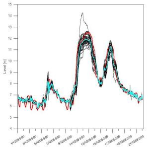
Figure 5.1: 2008 flood event computed without rainfall (Expt #1) where the red line is the observed and the blue is the mean of the 50 simulations, shown in black.
