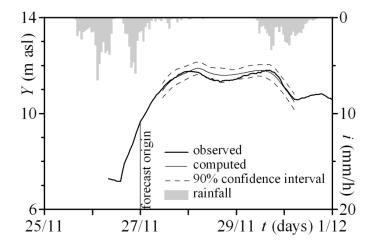
Figure 4.12: Comparison between the observed and 12h forecasted water levels from the TFF model for the November 2005 flood. Source: Napolitano et al. (2009).
