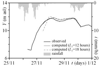
Figure 4.13: Comparison between the observed and forecasted water levels with two different lead times from the TFF model for the November 2005 flood. Source: Napolitano et al. (2009).
