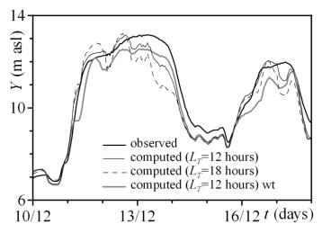
Figure 4.17: Comparison between observed and forecasted water levels with different lead times for the ANN model for the December 2008 flood. Source: Napolitano et al. (2009).
