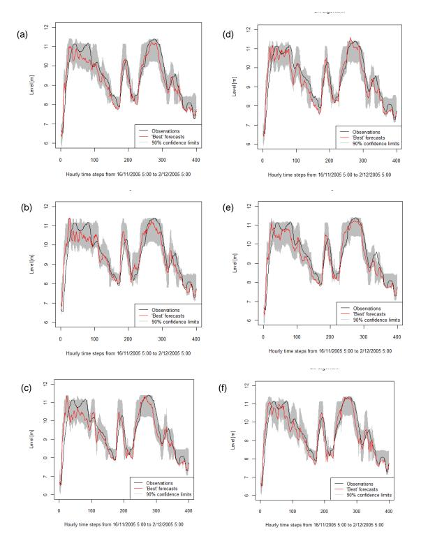
Figure 5.17: Confidence intervals (90%) shown in gray for a) to c) Expts # 29 to #31 and d) to f) Expts #32 to #34 for the 2005 flood event where the red line is the observed and the black line is the average of the simulations determined by the PI threshold method.
