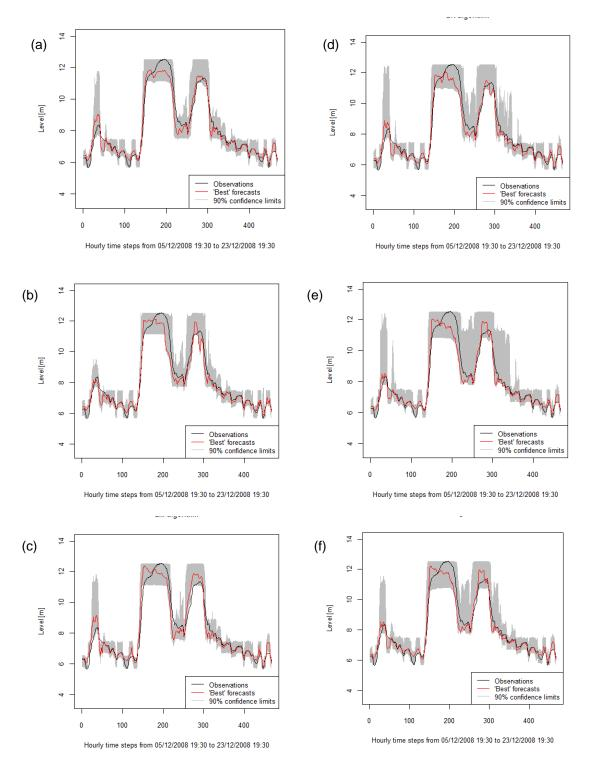
Figure 5.18: Confidence intervals (90%) shown in gray for a) to c) Expts # 35 to #37 and d) to f) Expts #38 to #40 for the 2008 flood event where the red line is the observed and the black line is the simulations determined by the AIC.
