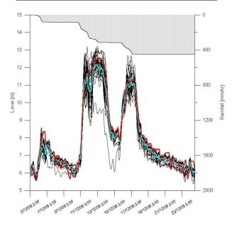
Figure 5.5: Results for Expt #8 for the 2008 flood event. The red line is the observed and the blue is the mean of the 50 simulations, which are shown individually in black. Cumulative rainfall is shown in grey at the top of the figure.
