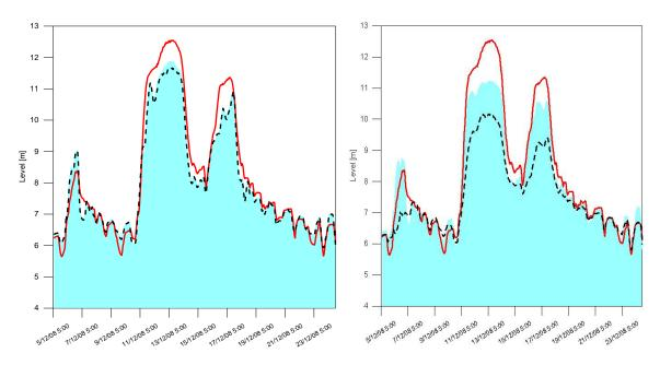
Figure 5.7: Results for a) Expts #13 and 14 and b) Expts #15 and 16 for the 2008 flood event. The red line is the observed, the dotted blue line is the MapStd method and the light blue filled in area is the MapMinMax method.
