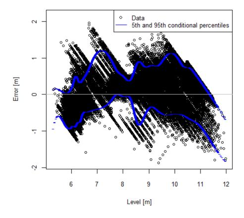
Figure 5.15: Quantile Regression with a spline of 25 degrees of freedom applied to Expt #18 for the error plotted againt the forecasted water levels
