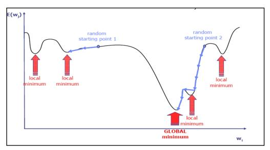
Figure 2.3: Local and global minima of errors
