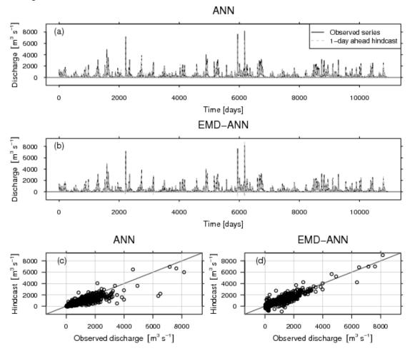
Figure 6.4: The Potomac River discharge time series of the test period along with 1-day ahead hindcasts obtained by (a) a simple ANN and (b) the EMD–ANN model. Scatterplots of the observed discharge vs hindcasts computed by (c) the ANN and (d) the EMD–ANN. Source: Napolitano et al. (2011).
