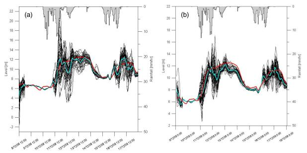
Figure 5.3: The results for (a) Expt#4 and (b) Expt #5 for a lead time of 12 hours for 2008 flood event. The red line is the observed, the blue is the average of the 50 simulations, which are shown in black, and observed rainfall is shown at the top of each figure in grey.
