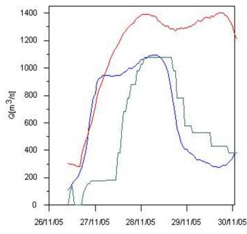
Figure 4.8: Observed discharge hydrographs flowing into the reservoir (in red), released from Corbara dam (blue), and at Ripetta gauging station (green) for the flood event that occurred in November 2005.
