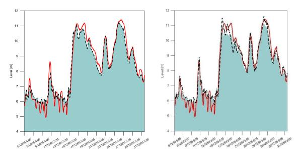
Figure 5.6: Results for a) Expts #9 and 10 and b) Expts #11 and 12 for the 2005 flood event. The red line is the observed, the dotted black line is the MapStd method and the light blue filled in area is the MapMinMax method.
