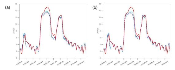
Figure 5.11 a) Expts # 35 to 37 and b) Expts #38 to 40 for the 2008 flood event where the red line is the observed, the dotted blue line is the LM algorithm, the light blue line is the BR algorithm and the gray line is the BFGS algorithm.
