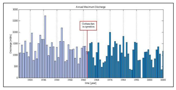
Figure 4.6: Annual maximum discharge at Ripetta gauging station in Rome.
