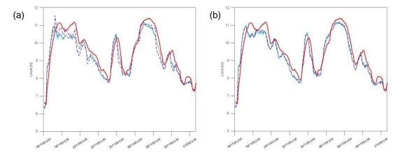
Figure 5.10: (a) Expts # 29 to 31 and b) Expts #32 to 34 for the 2005 flood event where the red line is the observed, the dotted blue line is the LM algorithm, the light blue line is the BR algorithm and the gray line is the BFGS algorithm.
