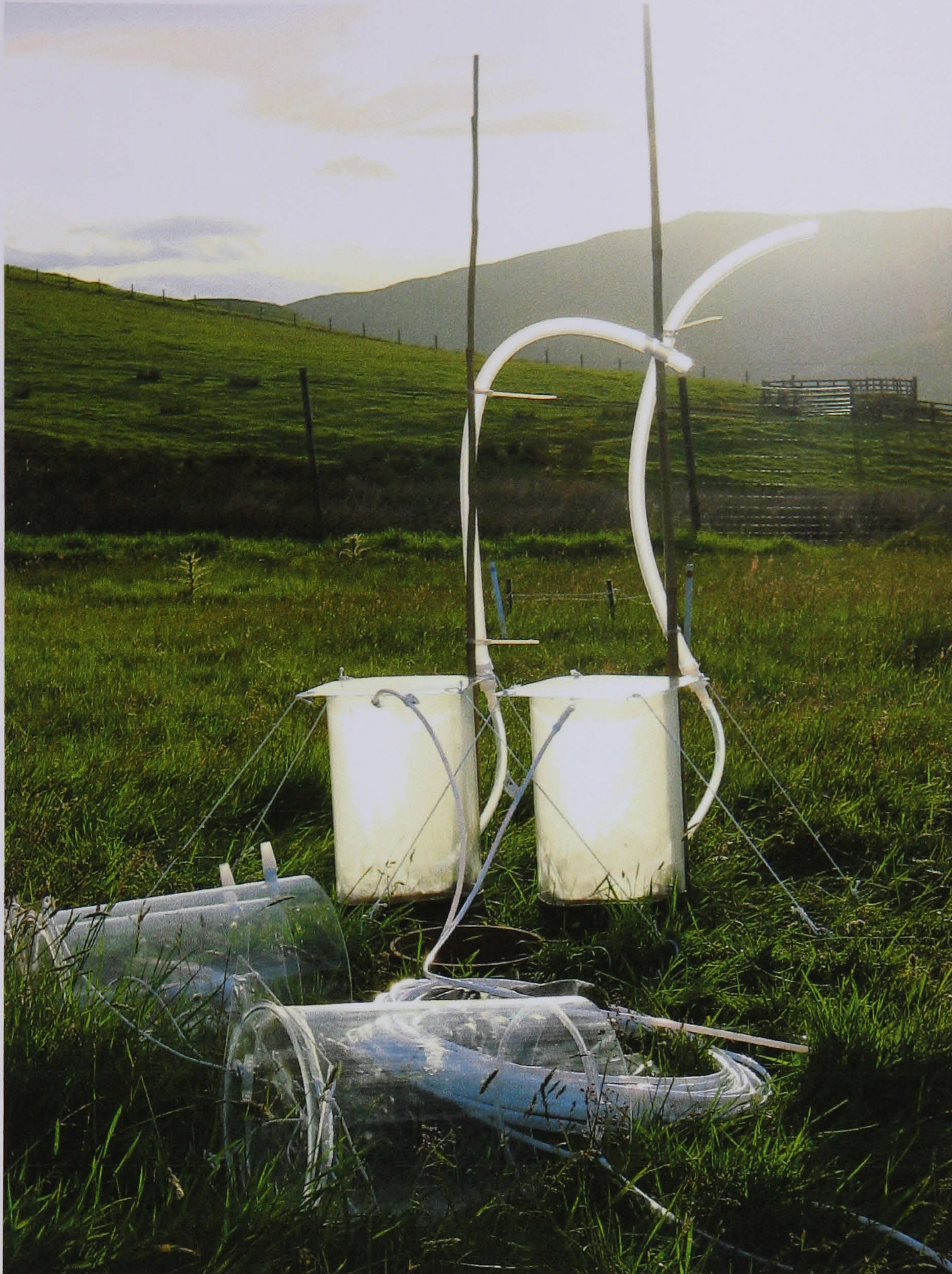
Plate 2 Photograph of the field site at Sourhope, showing the PTFE air sampling lines. Two chambers are shown lying on their sides, prior to being connected, as are the air intake pipes connected to two sampling chambers, prior to being covered with black bags. The plate is for demonstration purposes only and does not reflect the methodology in experiments where there was only one chamber per block.
