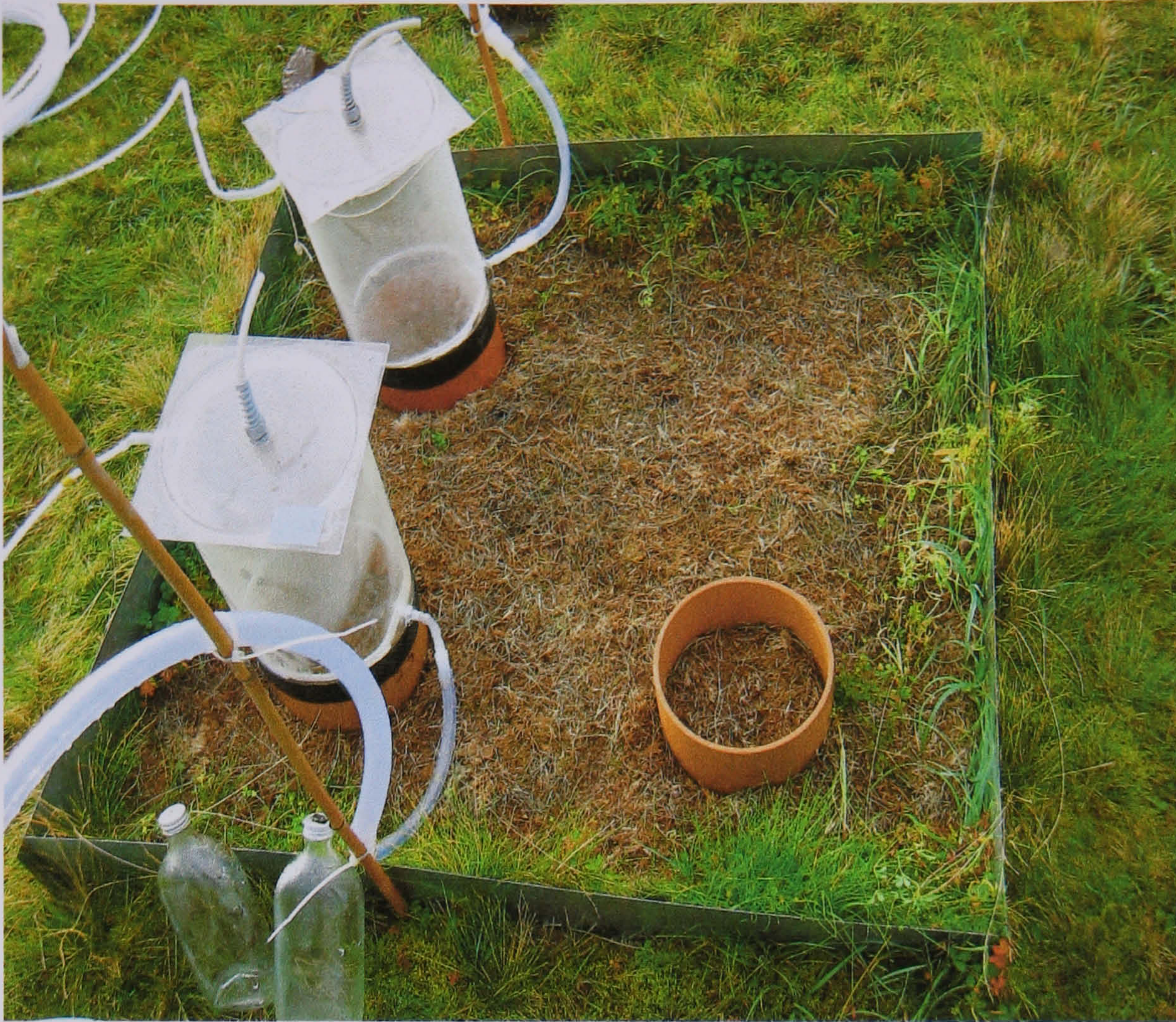
Plate 3 Photograph of the field site at Sourhope, showing a vegetation free plot in block 1, with the plastic collar inserted into the ground and two chambers connected to the air intake and PTFE pipes prior to being covered with black bags. This plate is for illustrative purposes only, since all the addition experiments used only one chamber per block.
