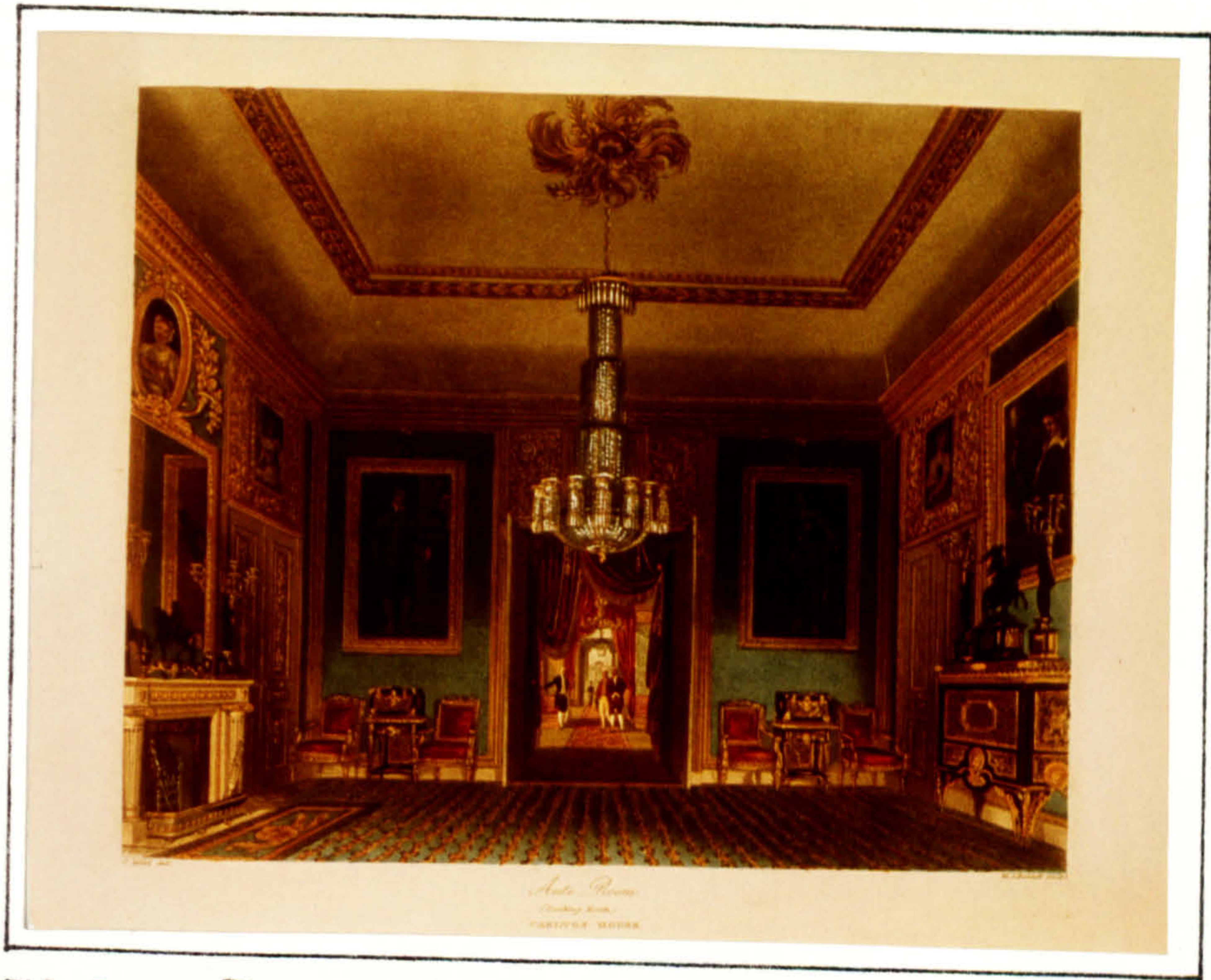
FIG. 26 ANTE-ROOM AT CARLTON HOUSE WITH WALLS DECORATED IN DISTEMPER MADE FROM BLUE VERDITER
