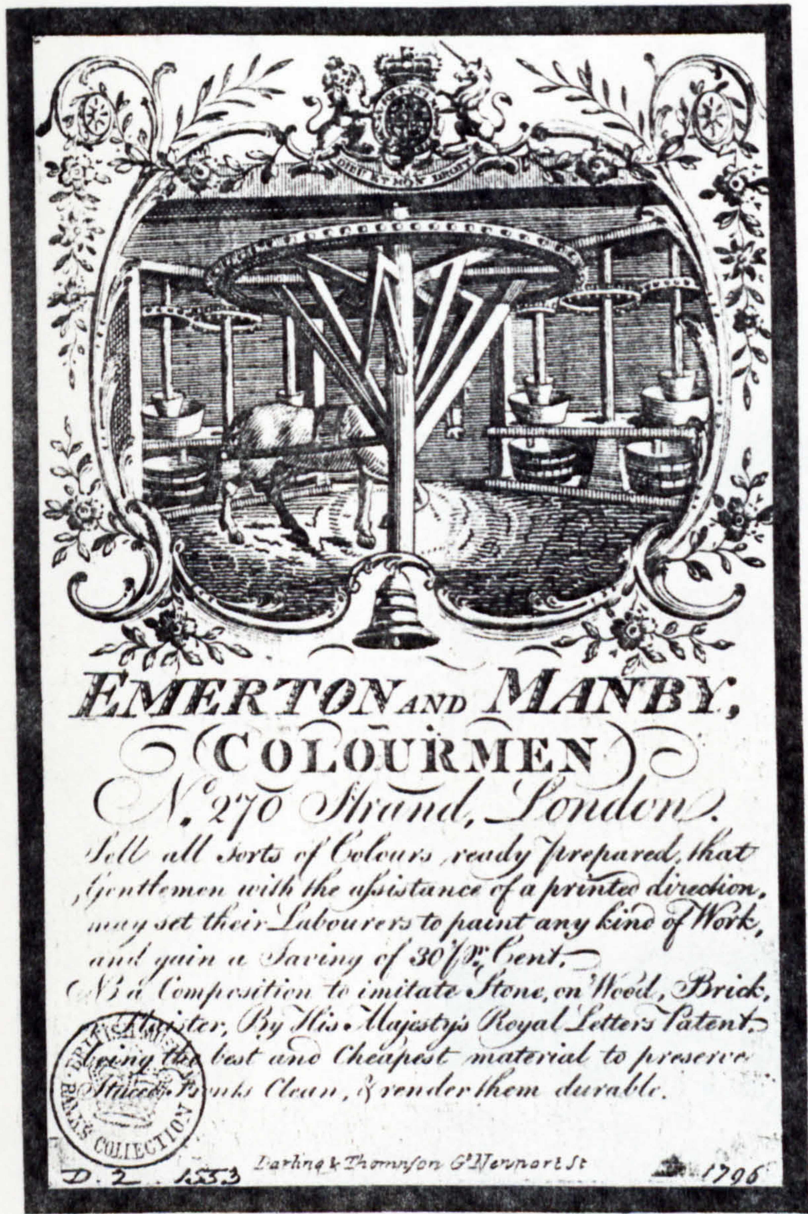
FIG. 8 EMERTON'S HORSE MILL FOR GRINDING PIGMENT INTO OIL
