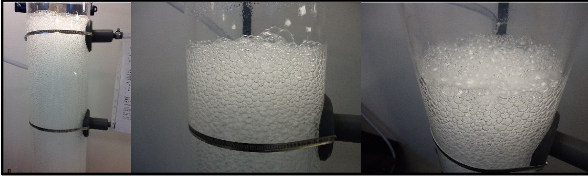
Figure 4.5: Left, froth in its optimum height (distance between belts is 30 cm). Middle, close view for the upper part of froth. Right, view for froth surface
