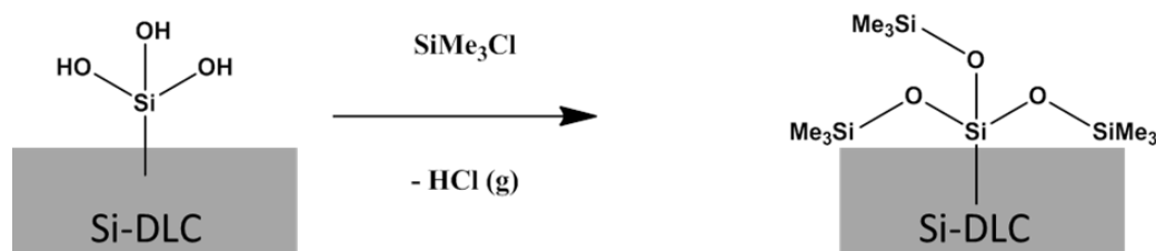
Figure 9-15 'Capping' of free -OH groups on the Si-DLC surface. Me represents the methyl, or CH 3 group.
