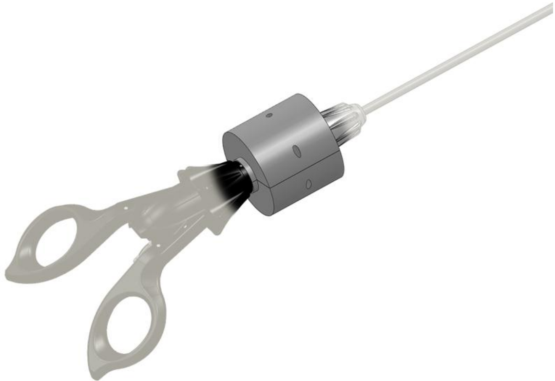
Figure 3.43: CAD of the redesigned instrumented grasper prototype, highlighting the location of instrumented module.
