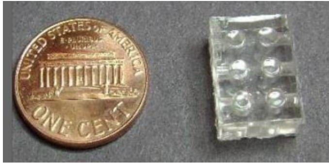
Figure 2.39: Pneumatic actuated balloon tactile display [199] .
