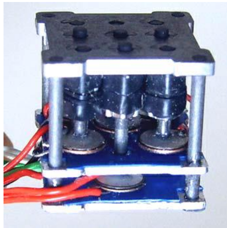
Figure 2.38: Actuator driven pins set in a tactile display [198] .
