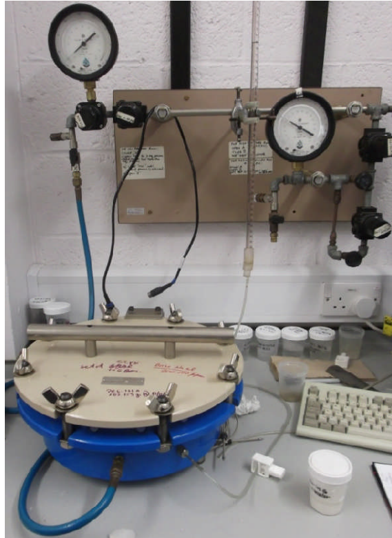
Figure 3.11 Air-Water porous plate apparatus
