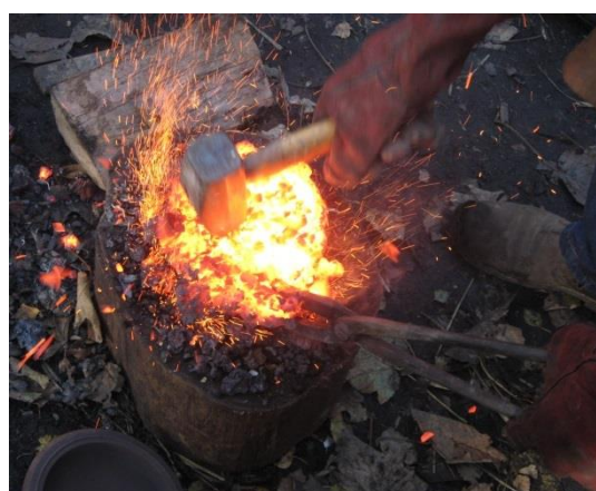
Figure 6.6 Clockwise from upper left: Plan of Experiment III Site A, Ecclesall Woods, Sheffield (image by author); image of experimental site with shaft furnace at centre being tapped, in foreground is the stump used for smithing, and to the right is a portion of the bellows utilised for forced draught (photograph by author); image of primary bloom smithing carried out directly after removing bloom from the shaft furnace (photograph by author); and image of two students processing the pelletised ore for the iron smelt by crushing with hammerstones (photograph courtesy of J. Karjalainen).
