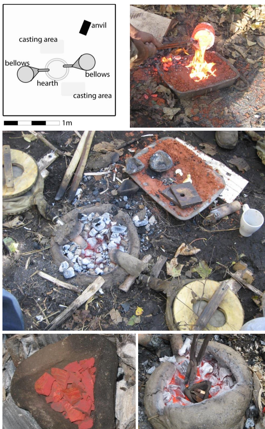
Figure 6.16 Clockwise from upper left: Plan of Experiment V Site B, Ecclesall Woods, Sheffield (image by author); image of copper casting (photograph courtesy of J. Karjalainen); image of hearth and two sets of single chambered bag bellows as well as the upper casting area with used and unused crucibles visible (photograph by author); image of crucible charged with pieces of copper-alloy being placed in the hearth (photograph by author; and image of cuprite in crucible ready for placement in hearth (photograph courtesy of J. Karjalainen).
