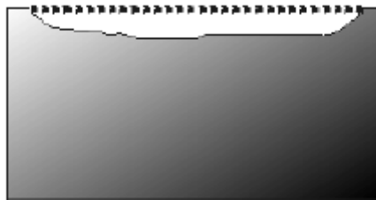
Figure 2.2: Schematic diagram of uniform corrosion ( http://corrosion-doctors.org/Forms-Uniform/uniform.htm )
