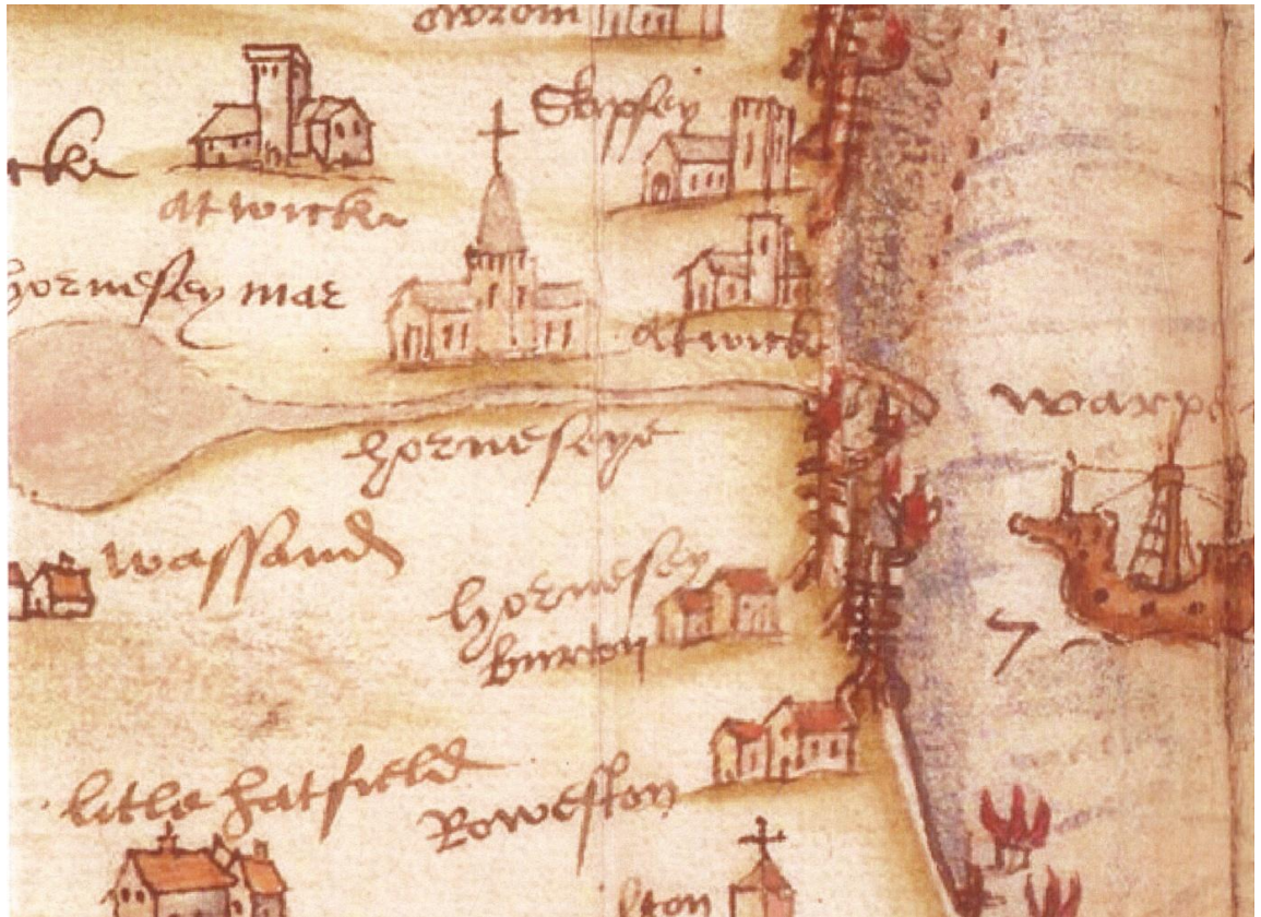
Figure 4, Extract of manuscript map of 1595 showing the pier at Hornsea in greater detail. There are distinct suggestions of a double pier arrangement with a large pier to the north of the stream and a smaller pier to the south. (British Library, Royal. MS. 18. D. 111, f.63)
