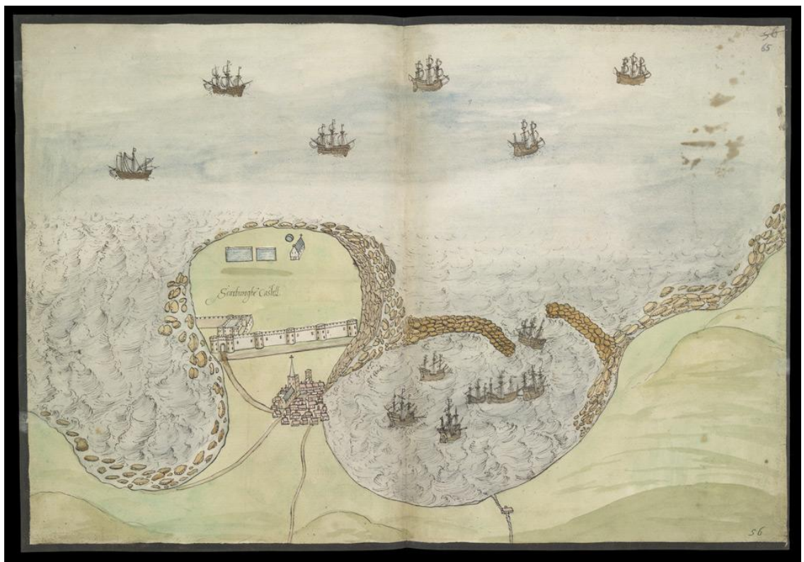
Figure 8, Twin pier system of stone, c.1595 (British Library, Royal MS. 18. D.III. f.65)
