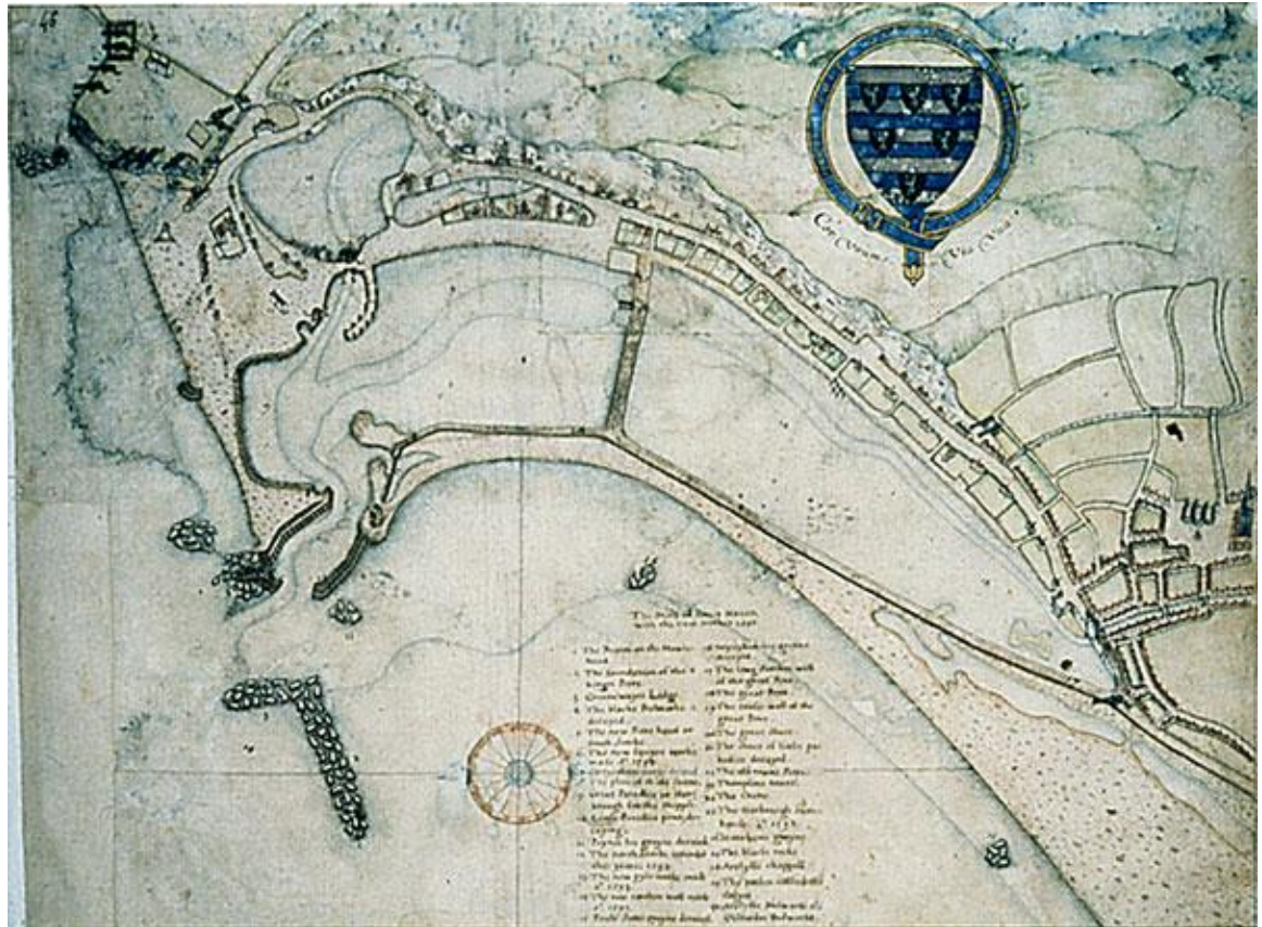
Figure 87, Dover harbour in 1595, by Thomas Digges. Controlled release of water via a sluice in the internal cross-wall of the harbour served to scour the lower basin and harbour mouth. North is to the right (British Library Cotton Augustus I.i.46)
