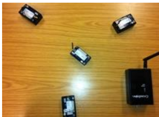
Fig. 4.2 Capture effect application environment, three senders, one receiver in the middle and a base-station.
