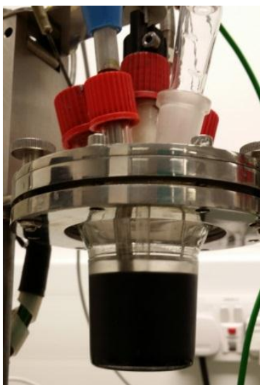
Figure 7.1 HEL Automate reactor vessel illustrating the dark colour solution that resulted upon addition of catalysts 4 and 5 to substrate 2 which prevented the use of on-line analytical techniques
