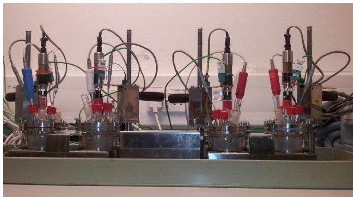
Figure 6.1 HEL Automate parallel overhead-stirred jacketed reactor system (30 ml scale) used to conduct determine the solubility curve of 4-rac mix -2 .
