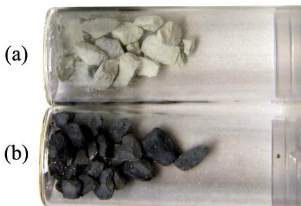
Figure 4.1 Colour change of MoO x source pellets after one evaporation: (a) fresh pellets and (b) pellets after one thermal evaporation.
