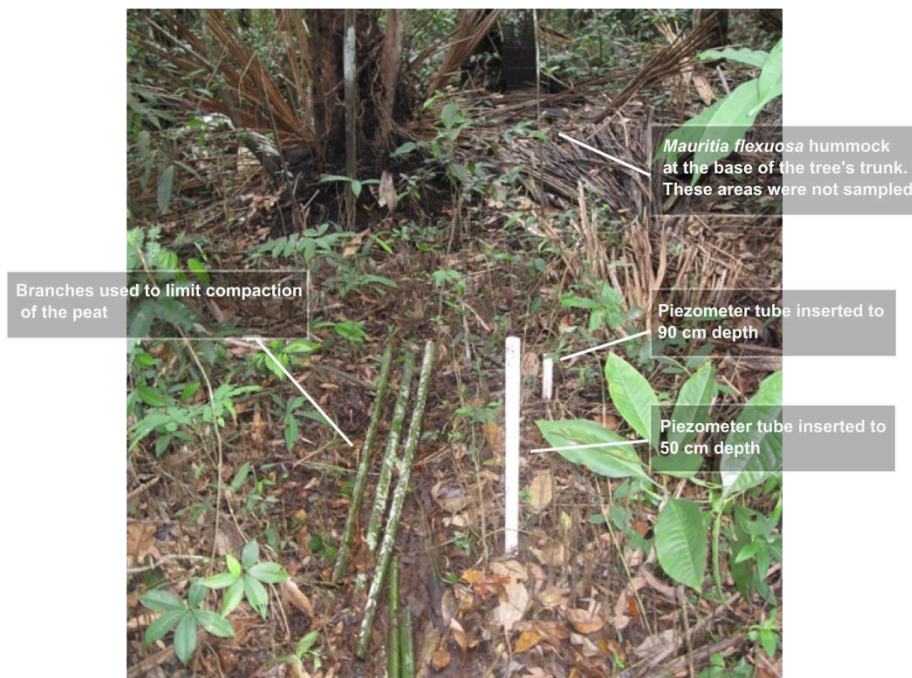
Figure 4.1: Photograph showing piezometer tubes installed one metre apart at Quistococha peatland. Branches were used to limit compaction of the peat in adjacent areas by the operator during the insertion of the tubes. A Mauritia flexuosa hummock can be seen in the background formed from large palmate leaves; this kind of microtopography was avoided during sampling.
