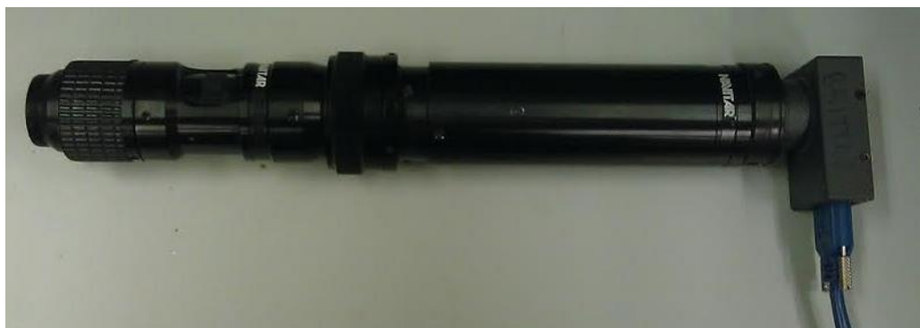
Figure 3.11. Photograph of the Pixelink 5.3 MegaPixel camera with Navitar lens and lens adapter
