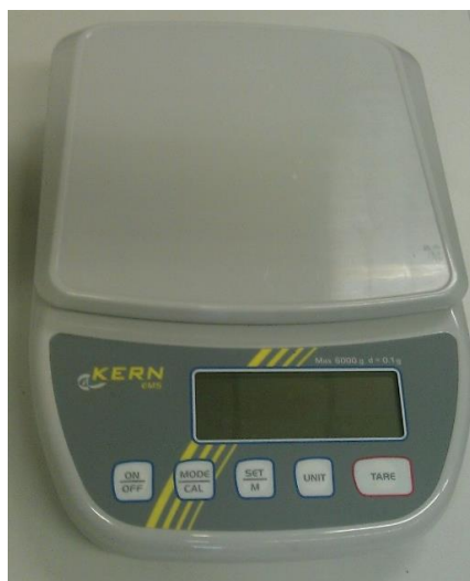
Figure 3.13. Photograph of Kern EMS 6K0.1 mass balance used to measure mass of water and MEA
