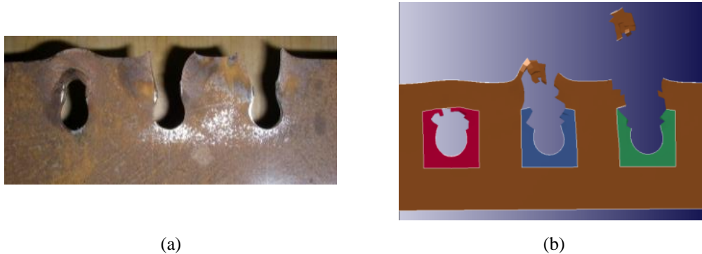
Figure 5-23 Final deformation of beam web (a) Experiments (b) Ls-Dyna
