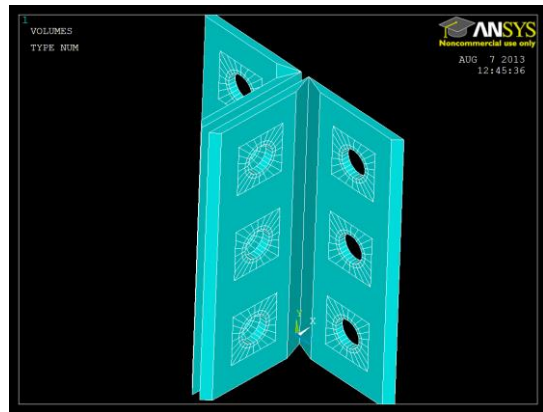
(a) (b) Figure 4-32 (a) Angles with square holes (b) Angles with the bolt holes
