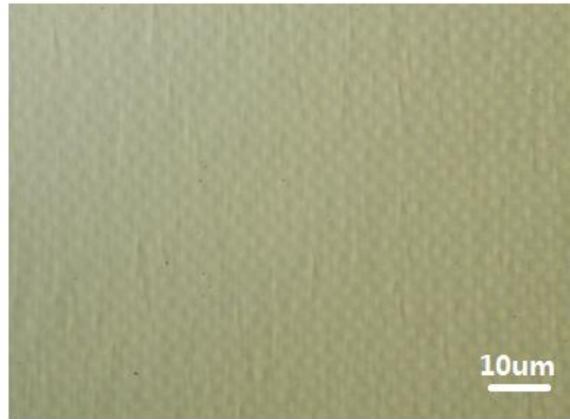
Fig. 6.8: Optical microscopy image of overgrown semi-polar GaN.
