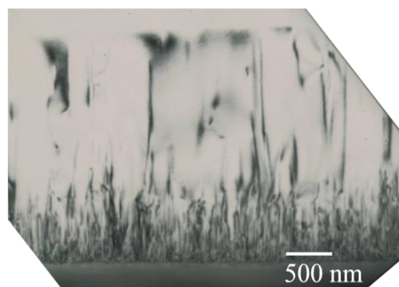
Fig. 3.8: An example TEM image measured by Phillips EM 430 of GaN grown on our porous AlN buffer by our group.
