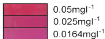
Figure 4-6 a colour map of three different dye concentrations within tank as seen in the results section.
