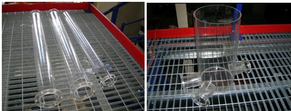
Figure 23 - Examples of scaled pipes on the left (a) and junction manhole on the right (b).
