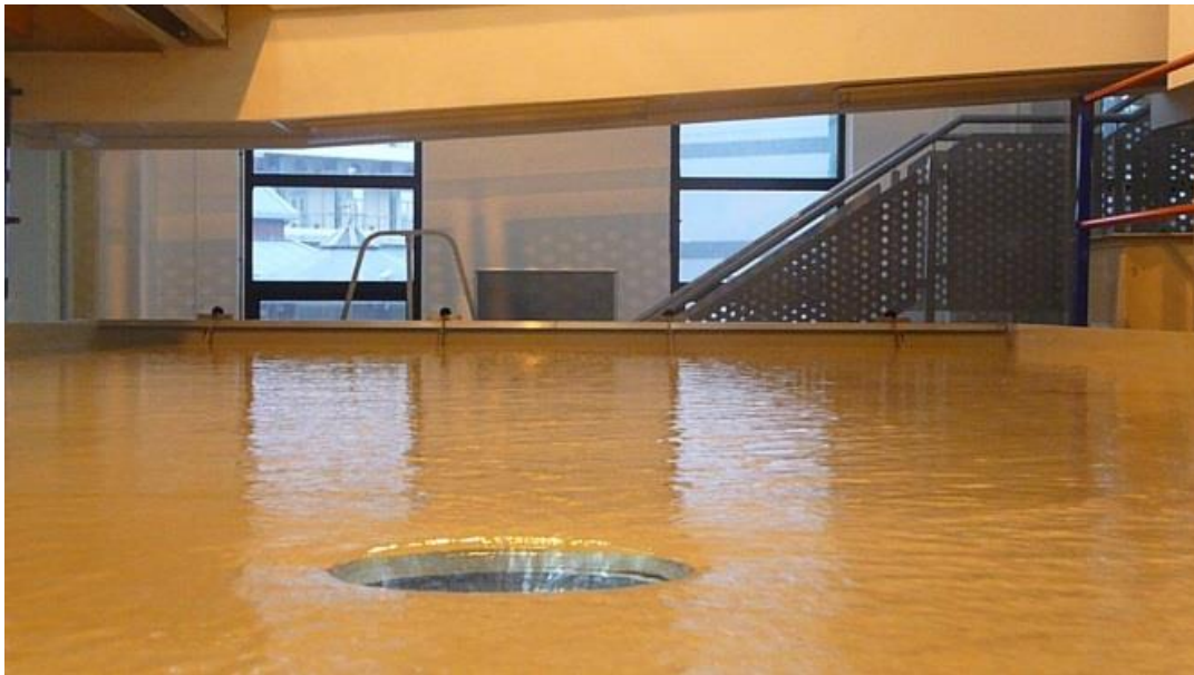
Figure 97– An example of surface to sewer exchange reproduced within the experimental facility.
