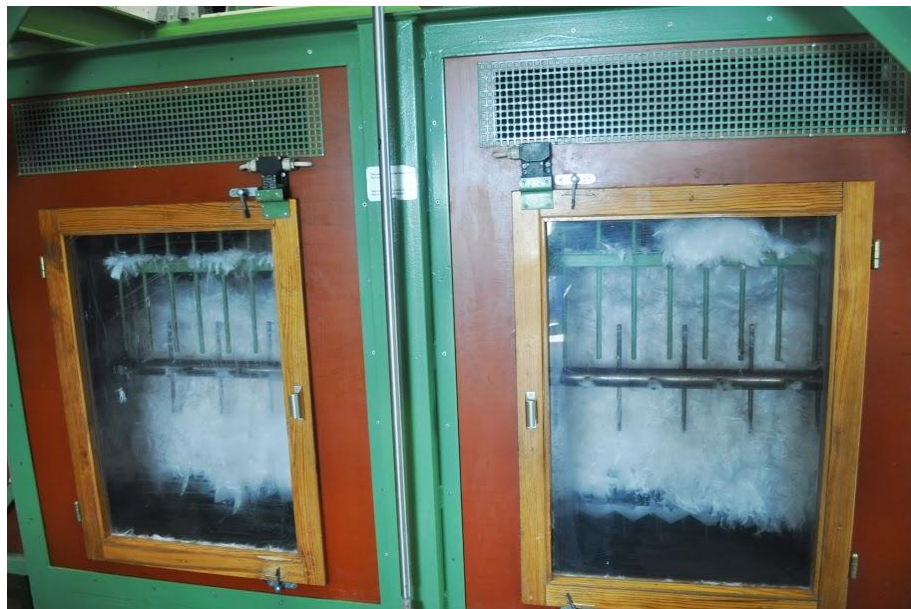
Figure 1-7 – drying of washed down and feathers (Taken at Peter Kohl Industries, Germany, 13 th July 2012)
