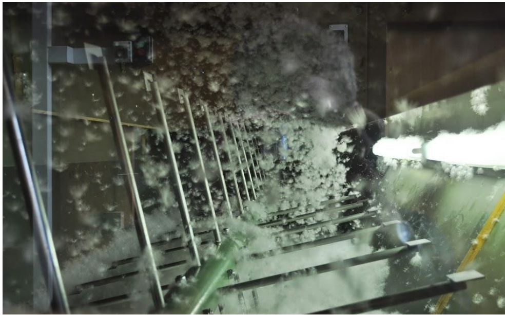
Figure 1-8 – sorting of down and feathers in air currents (Taken at Peter Kohl Industries, Germany, 13 th July 2012)
