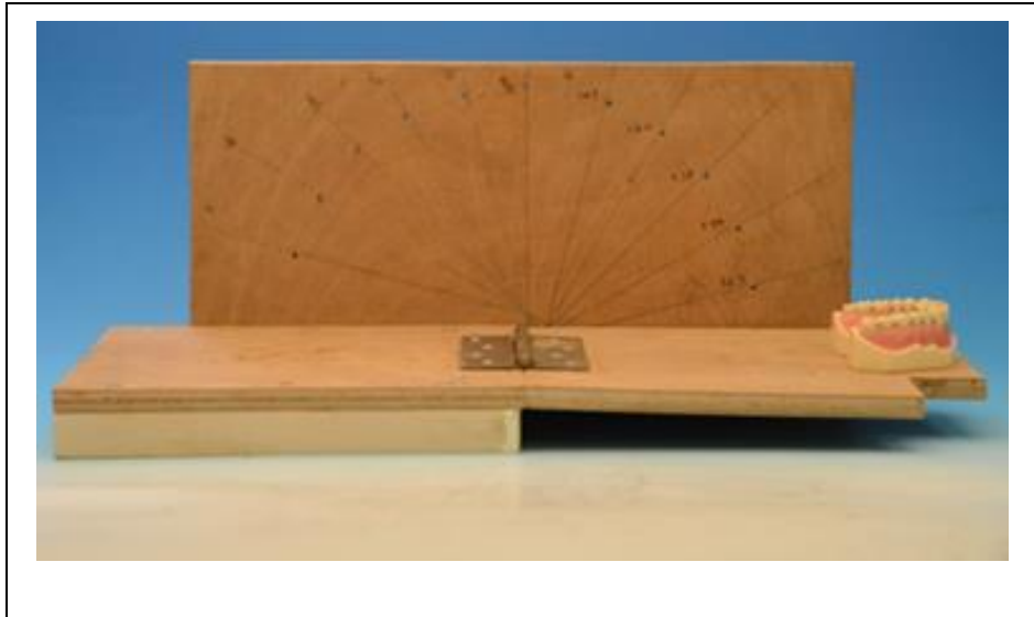
Figure 6.1: Device for simulating tooth angulation in the patient mouth
