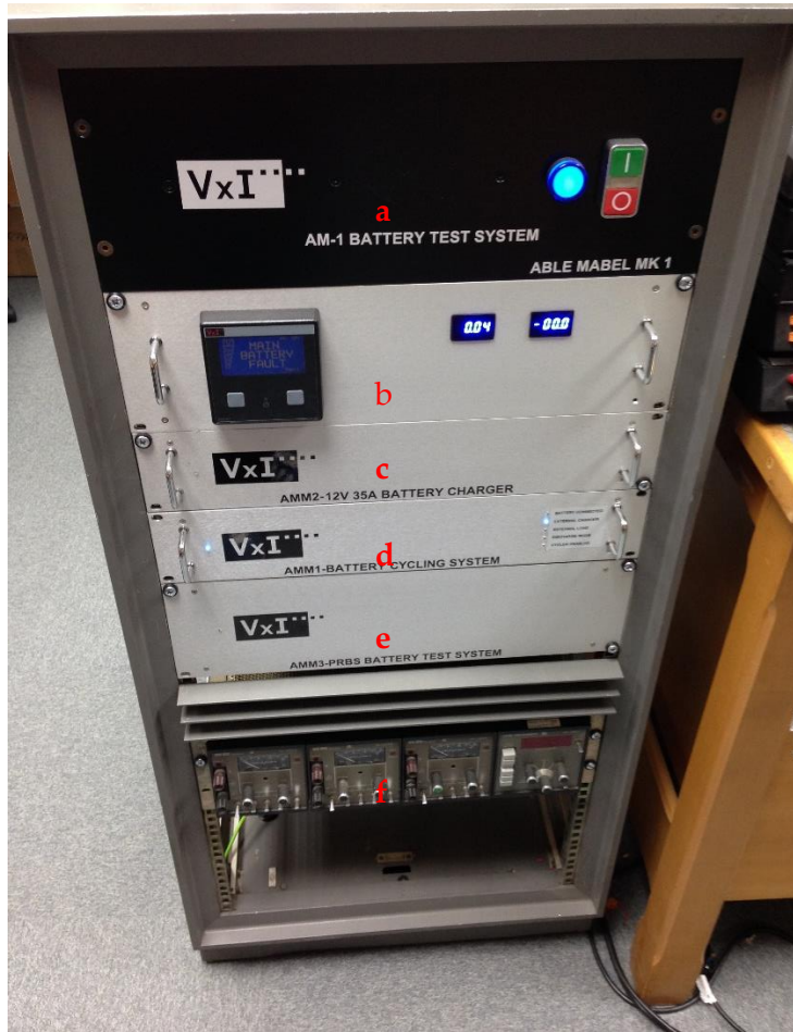
Figure 169. AM-1 test system photograph showing installed modules and rear interconnectivity
