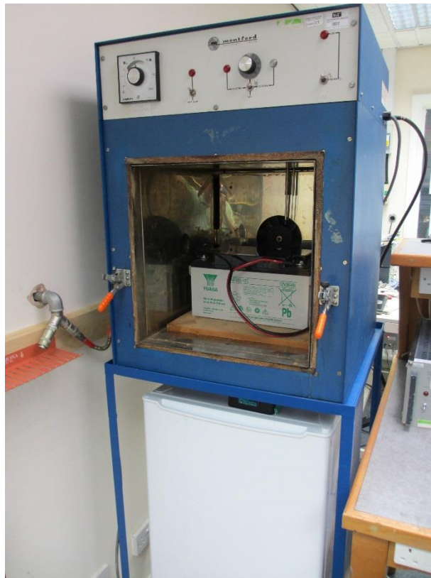
Figure 99. Test battery in Montford environmental chamber
