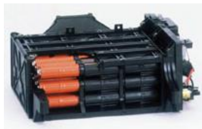
Figure 12. Honda Insight NiMH battery pack (image courtesy Bumblebee Batteries LLC)
