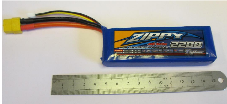
Figure 15. Lithium Polymer radio controlled model battery (photograph by author)
