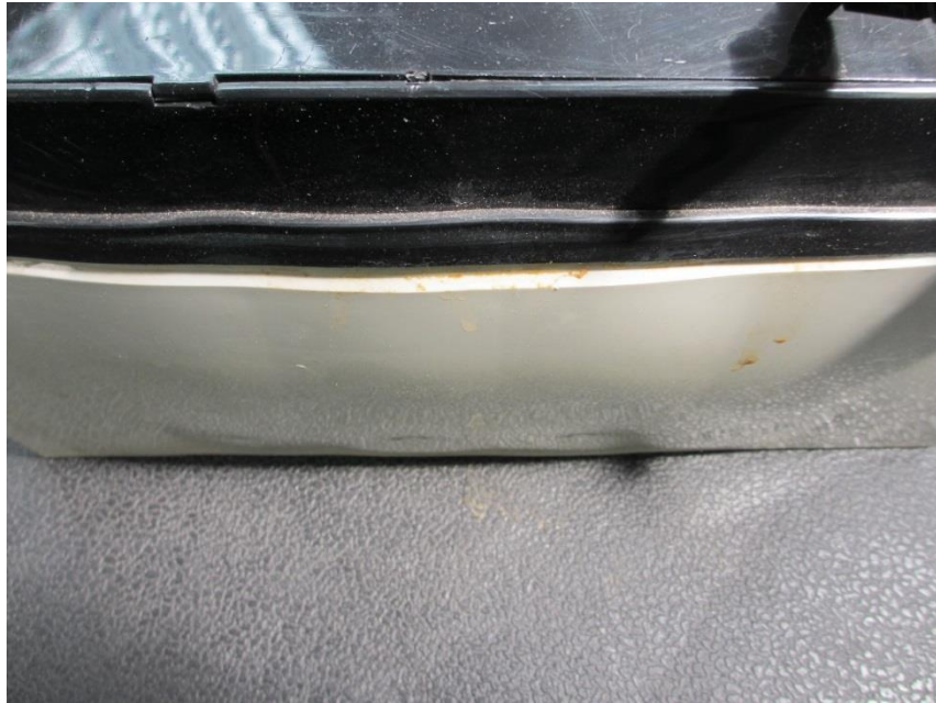
Figure 151. Case distortion of the battery during the elevated temperature tests
