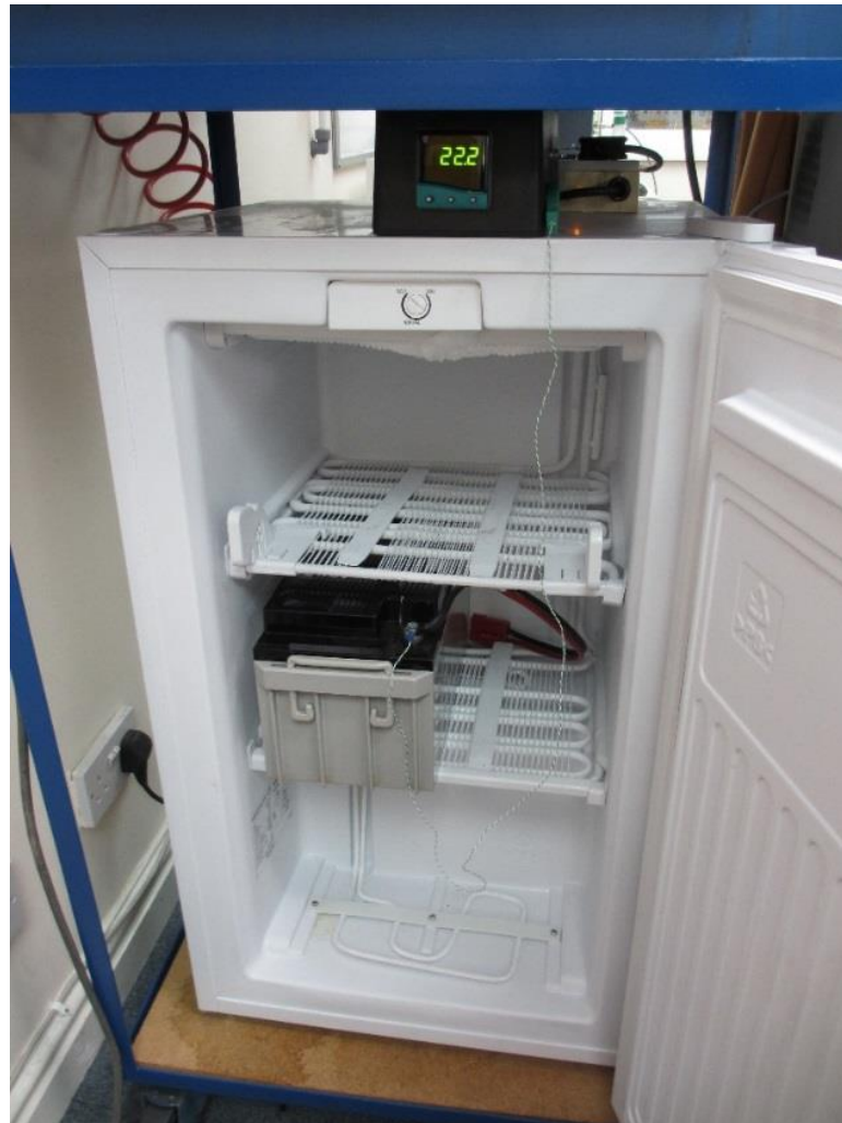
Figure 184. (a) Photograph of extended low temperature chamber, and (b) battery in situ within the chamber with thermocouple attached
