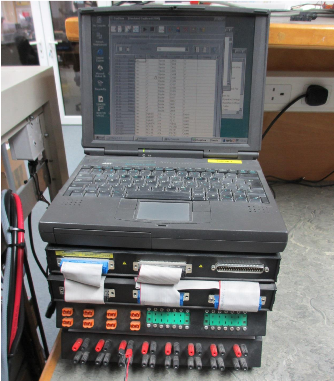
Figure 168. IOTech Daqbook 200 data acquisition system used for the high frequency tests
