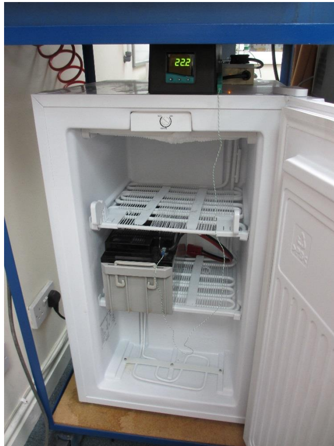
Figure 101. Test battery in low temperature chamber
