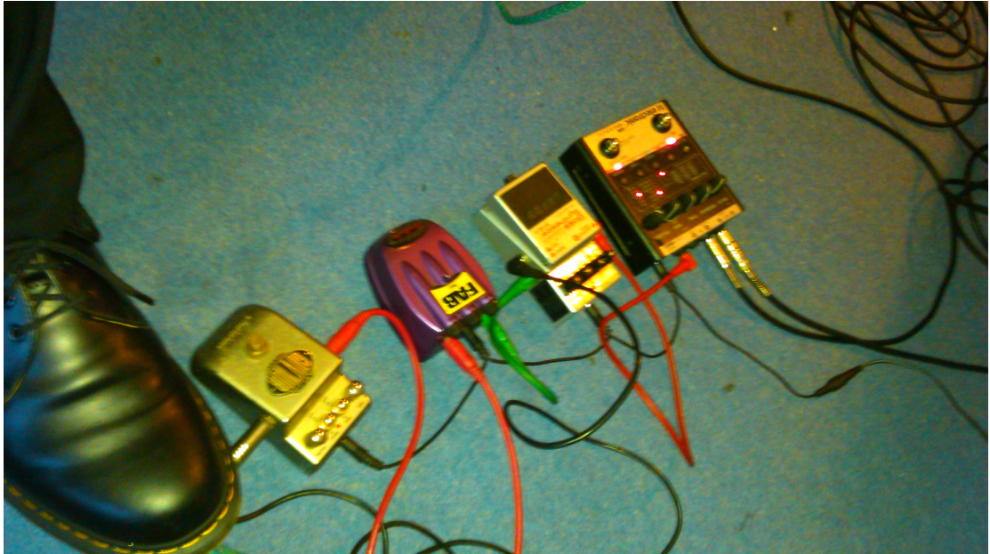
Figure 6 Effects chain for bass recording ( Song for Aberfan and Sense(or) ). From left to right: Marshall Guvnor distortion, Danelectro FAB fuzz pedal, Boss SYB-5 bass synthesiser, TC Electronics Delay ND-1 Nova Delay. The signal was then fed into a bass amplifier, which was recorded using a AKG D-112, and also fed to the instrument input on the Focusrite ISA pre-amp.
