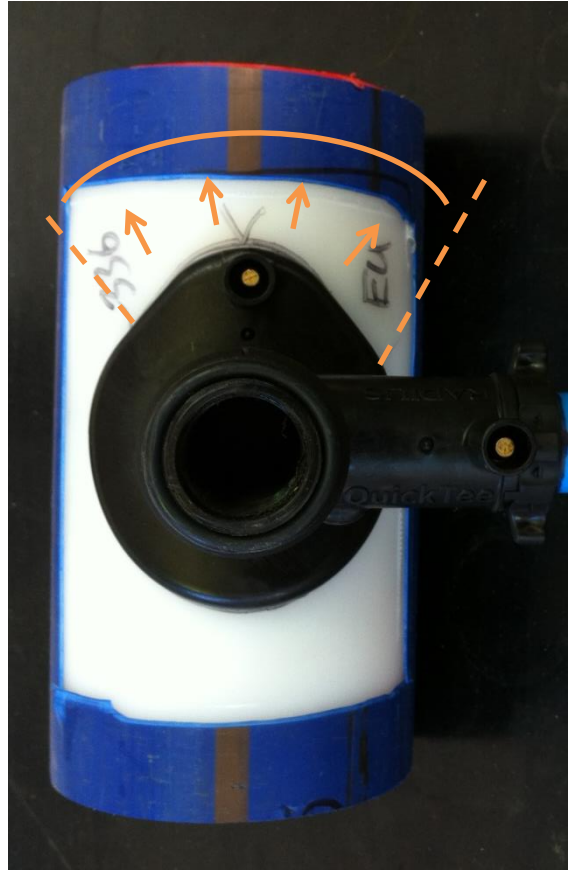
Figure 6-61 Specimen EU showing leak path area and direction
