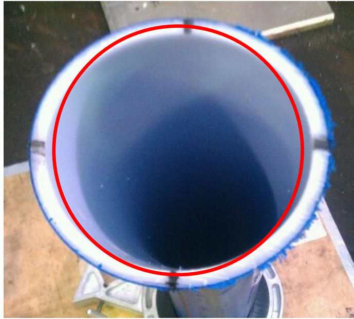
Figure 1-13 Ovality on a Ø180 mm PE pipe
