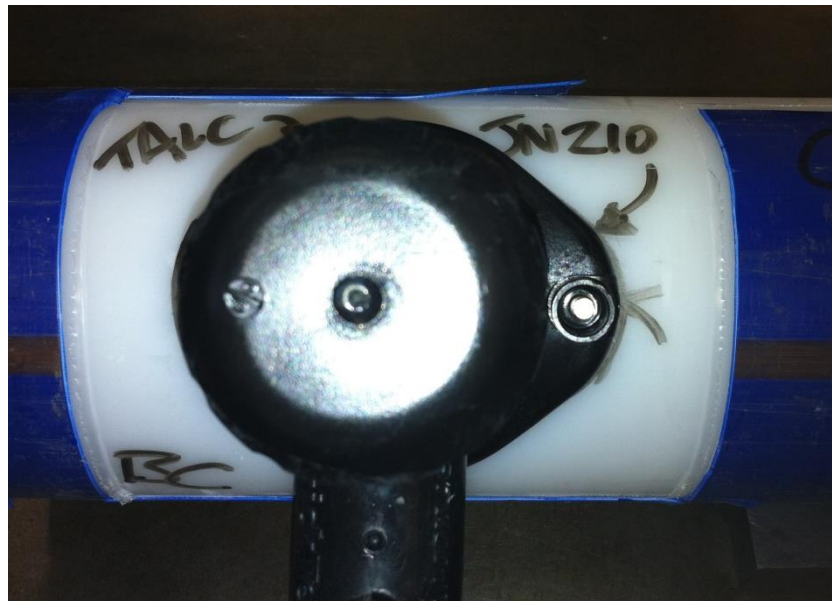
Figure 4-8 Electrofusion tapping without lateral shift (top view)
