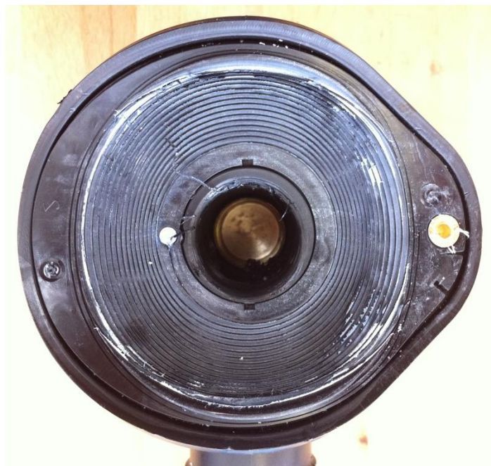
Figure 5-14 Specimen X tapping tee (removed)
