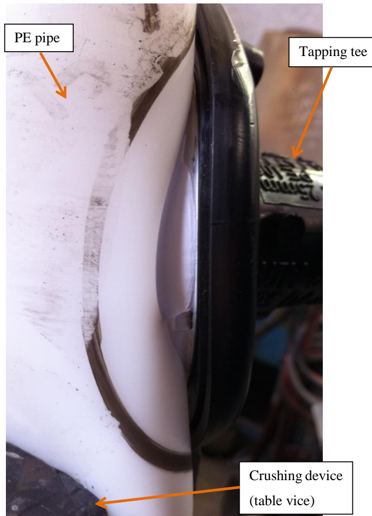
Figure 5-3 Post-crush of 'perfect' specimen
