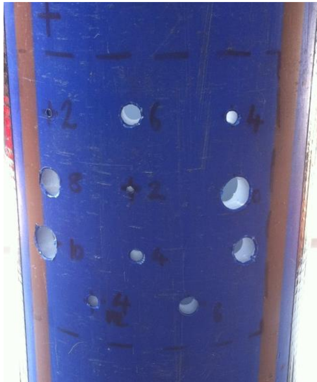
Figure 6-29 Ø110 mm pipe with holes drilled
