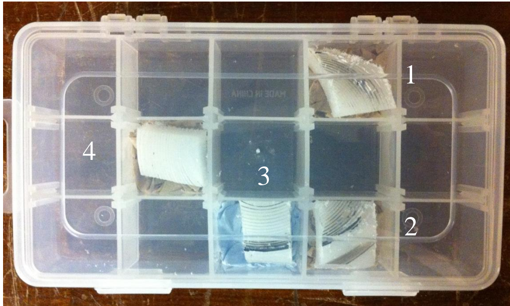
Figure 5-17 Specimen X samples for SEM
