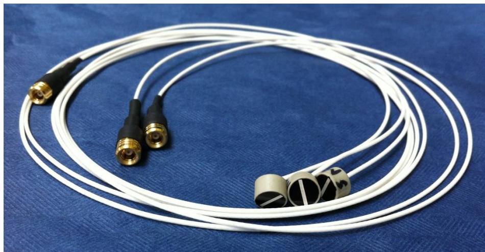
Figure 6-48 Individual ultrasound sensors
