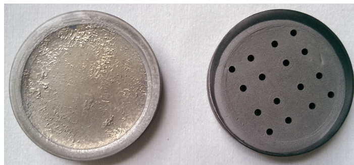
Figure 4.4: Image of a standard (left) and composite (right) HiTUS target.
