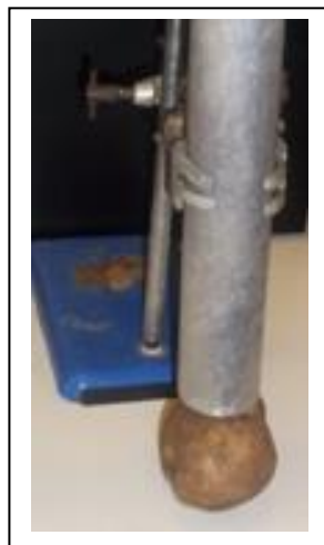
Figure 2.2 Aluminium guide tube for assessment of severe bruising using the falling bolt method
