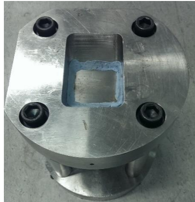
Figure 9.7 Loading Frame and Scanning Window
