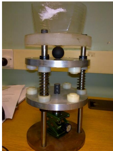
Figure 5.9 Loading Frame for Low Load Test
