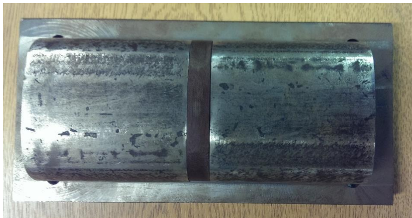
Figure 9.6 Endpost with Rail Sections
