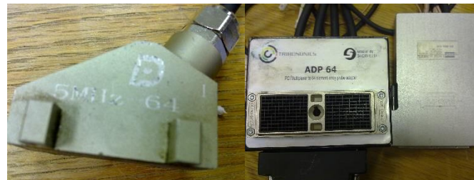
Figure 8.2 Ultrasonic Scanning Array and Multiplexor
