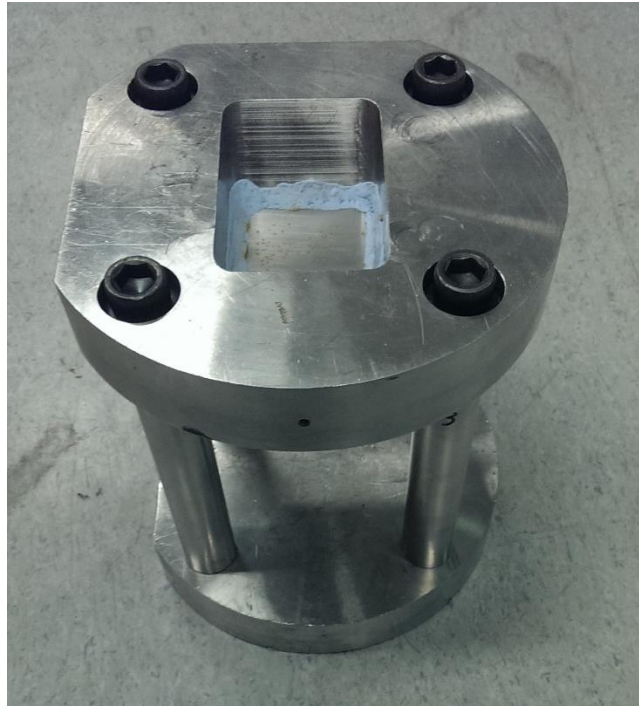
Figure 5.8 Loading Frame for High Load Test
