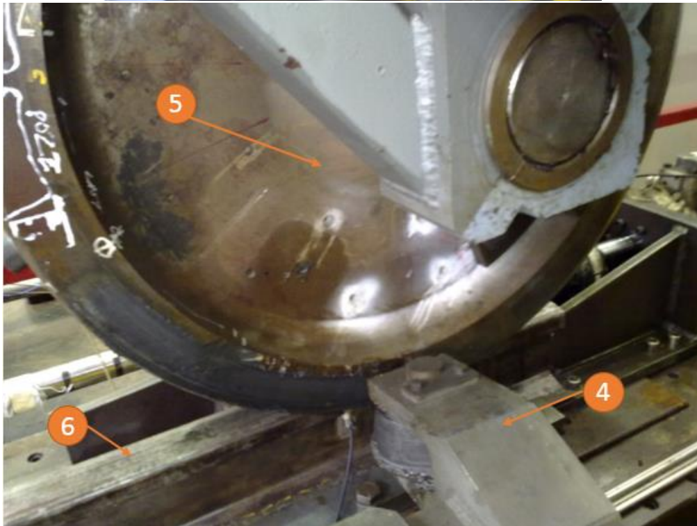
Figure 8.1 Full Scale Wheel/Rail Wear Test Rig (1: Vertical actuator; 2: loading frame; 3: Longitudinal Driving System; 4: Lateral Ram; 5: Wheel; 6: Rail)
