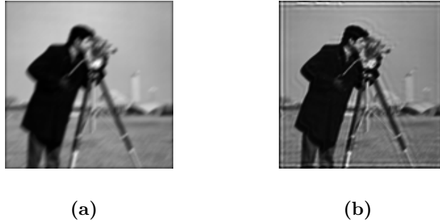
Figure 2.4: The boundary conditions problem in image restoration. (a) presents the blurred image using the linear motion filter of size 5 \times 5 and angle 45^\circ . (b) is the restored image using a Matlab built-in function, showing oscillations at its border.
