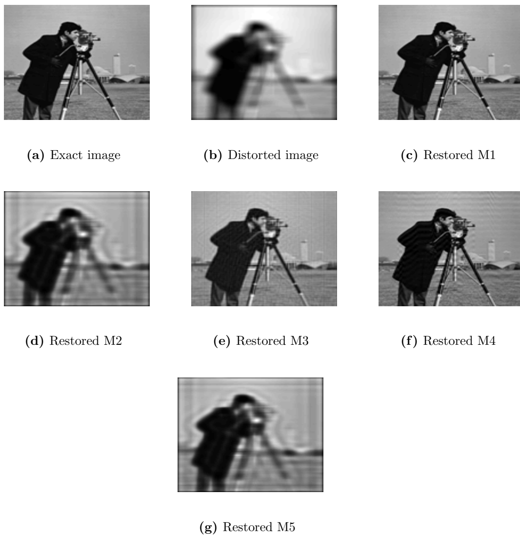
Figure 9.5: Image restoration using five deblurring methods of Cameraman–image presented in Example 9.3: (a) the original image; (b) the distorted image; (c) the proposed method using Method 1 as described in Chapter 7; (d) Lucy-Richardson; (e) regularised filter; (f) Wiener filter; (g) maximum likelihood.
