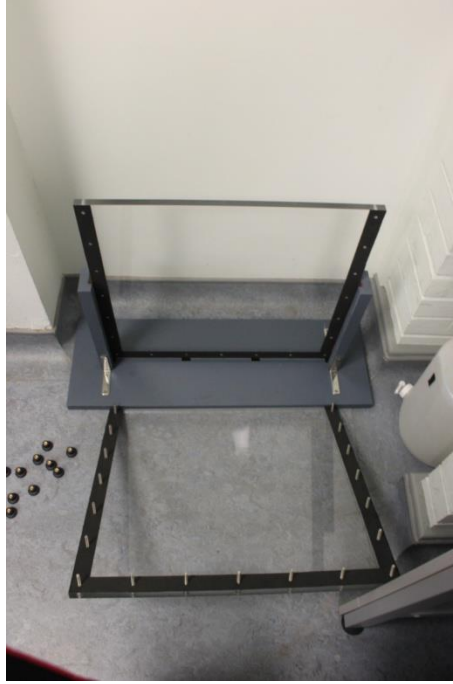
Figure 6.1.3: Revised, openable Hele-Shaw cell design
