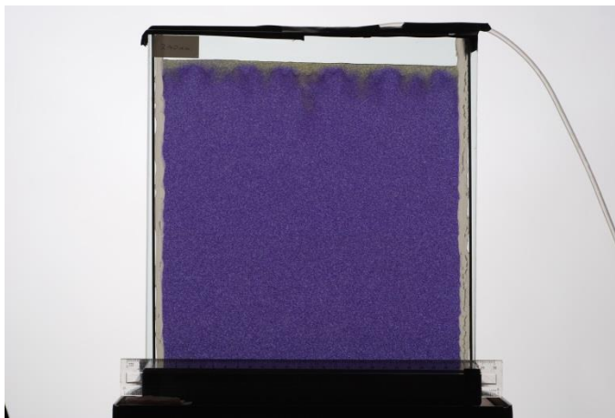
Figure 6.1.2: Original Hele-Shaw cell design
