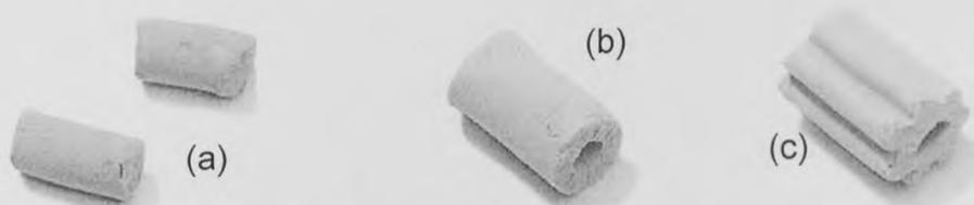
**Figure 12.1:** Main catalyst shapes. a) pellet type catalyst, b) ring type catalyst, c) ribbed or daisy type[99]
