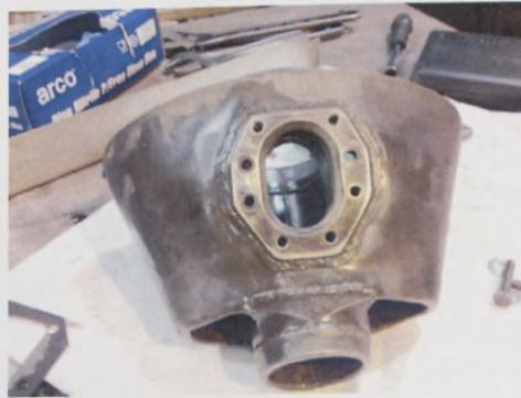
**Figure 7.3:** a) The cylindrical casing that houses the liner. b) A common Olympus diffuser and the place where the fuel injector mounts.
