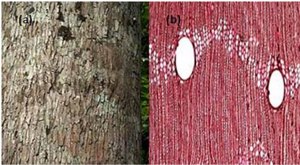
Figure 3-4: Photographic and SEM images of Terminalia superba showing (a) the bark (b) the wood in transverse section[141].
