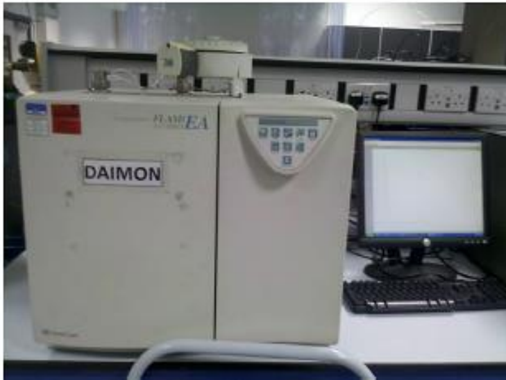
Figure 3-14: CE Instruments Flash EA 1112 Series elemental analyser.
