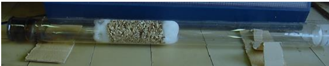
Figure 3-23: Image showing the positioning of the sample inside the reactor tube.
