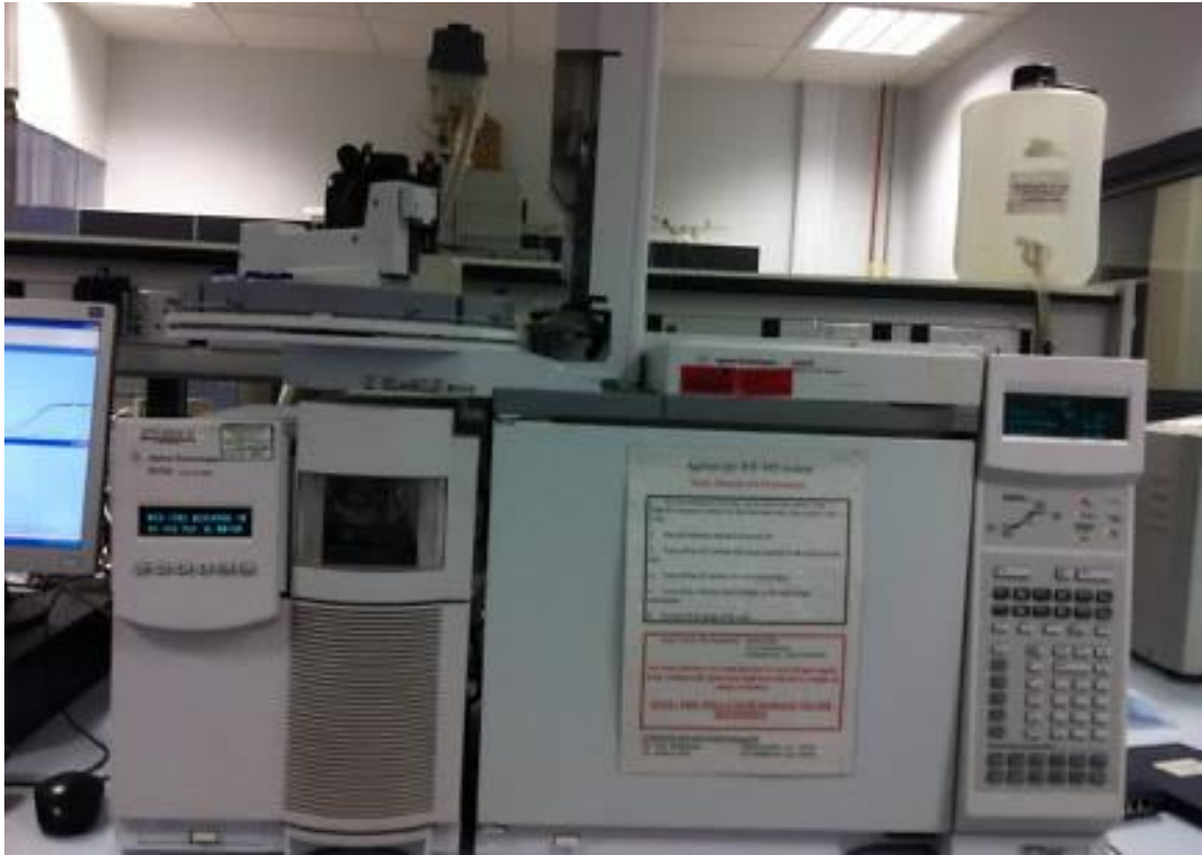
Figure 3-28: Agilent 7683 series auto sampler with Agilent 6890N Gas Chromatograph and Agilent 5975 Inert XL Mass Selective Detector.
