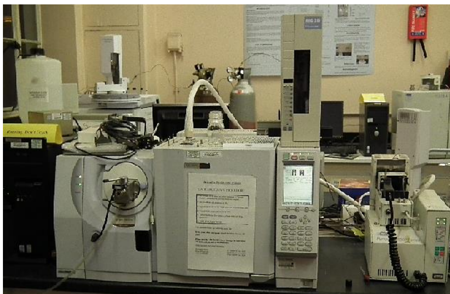
Figure 3-19: A CDS 1000 Pyroprobe with HP 5890 series II Gas Chromatograph.
