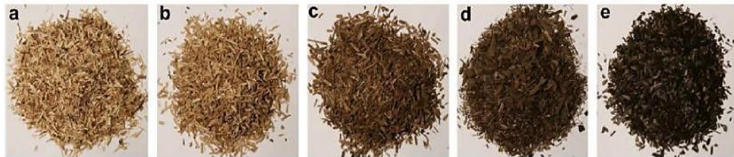
Figure 2-25: Images of willow: a) untreated; b) low temperature, short residence time; c) low temperature, long residence time; d) high temperature; short residence time; e) high temperature, long residence time [93].
