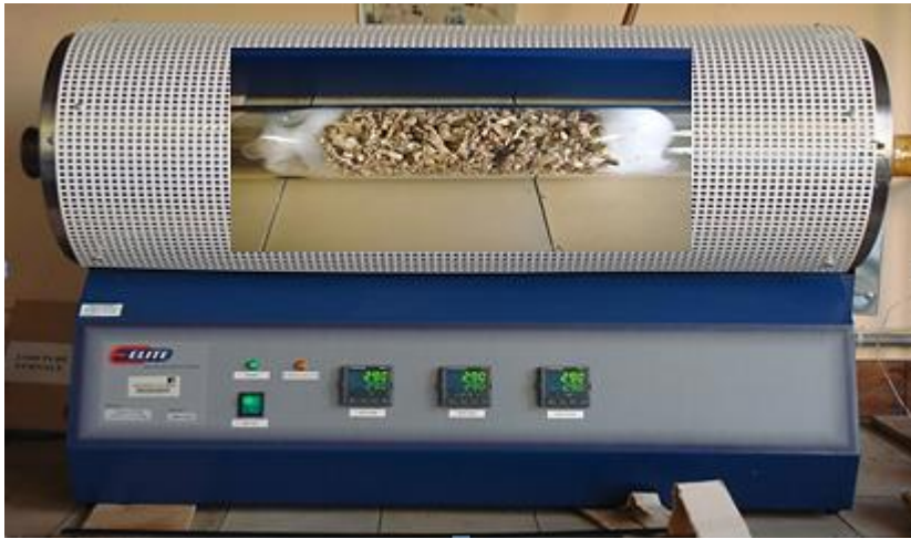
Figure 3-21: Torrefaction rig with a three temperature zone.
