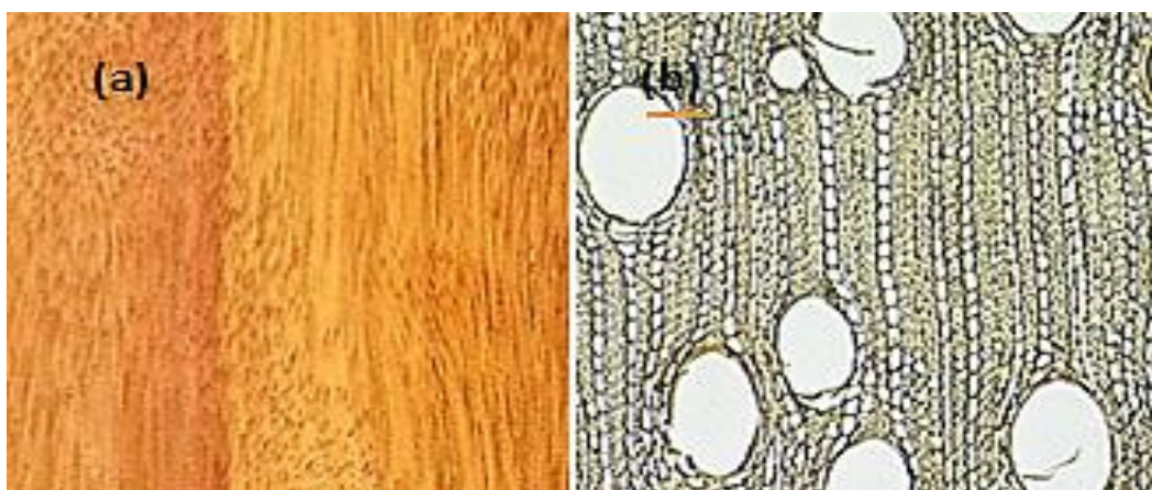
Figure 3-6: SEM images of Nauclea Diderrichii showing (a) wood surface (b) transverse section [148].
