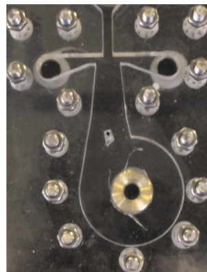
Photo showing position of splitter after adjustment to promote stability.
