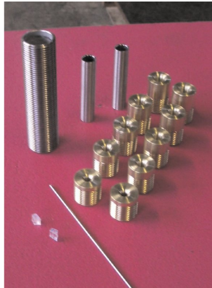
Accessories: supply and control pipes, splitters and outlet nozzles
