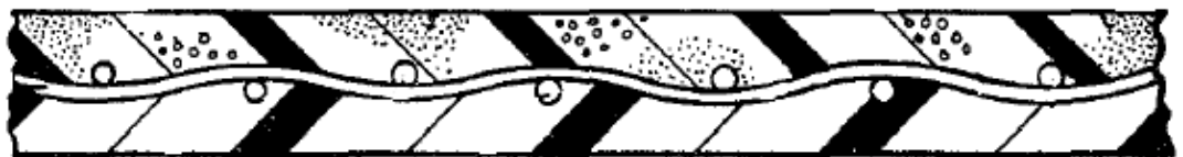
Figure 2-26. Microcapsules, containing lubricant, fully embedded within a surface which is released as wear occurs [101].
