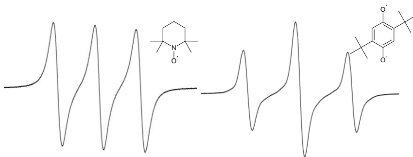
Figure 6. EPR spectra of TEMPO (Left) and 2,5 – di-tert-butyl semiquinone(Right)
