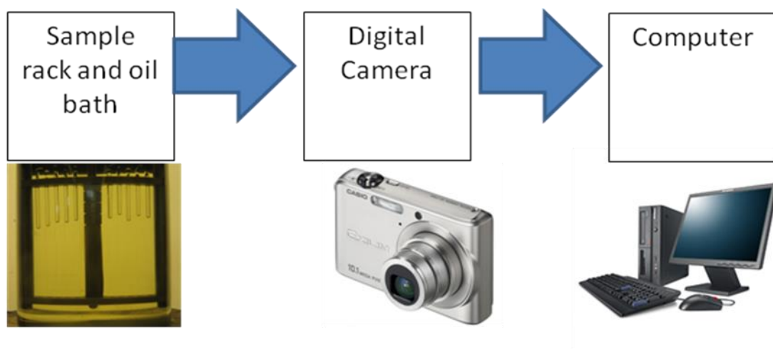
Scheme 22. Schematic of the small scale, automated dilatometry setup, developed to determine the onset of polymerisation after inhibition or retardation.
