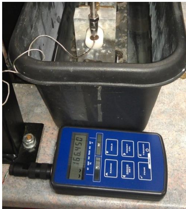
Figure 8-12: Force sensor device
