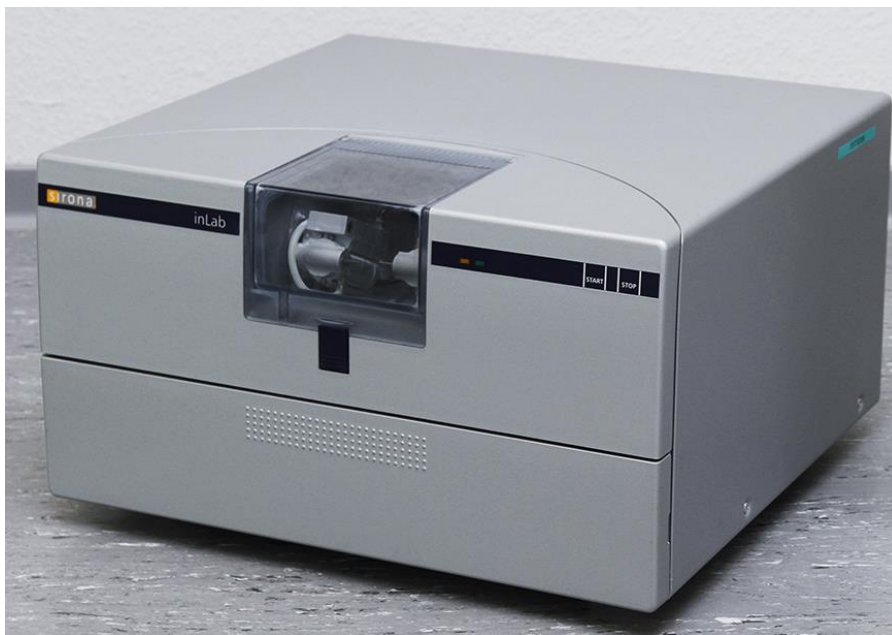
Figure 5-16: CEREC InLab CAD/CAM machine
