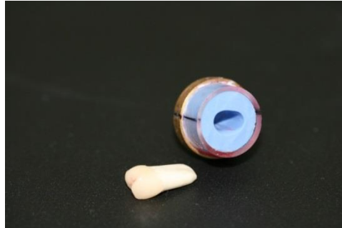
Figure 5-18: Alignment of the sample in the Micro CT scanner
