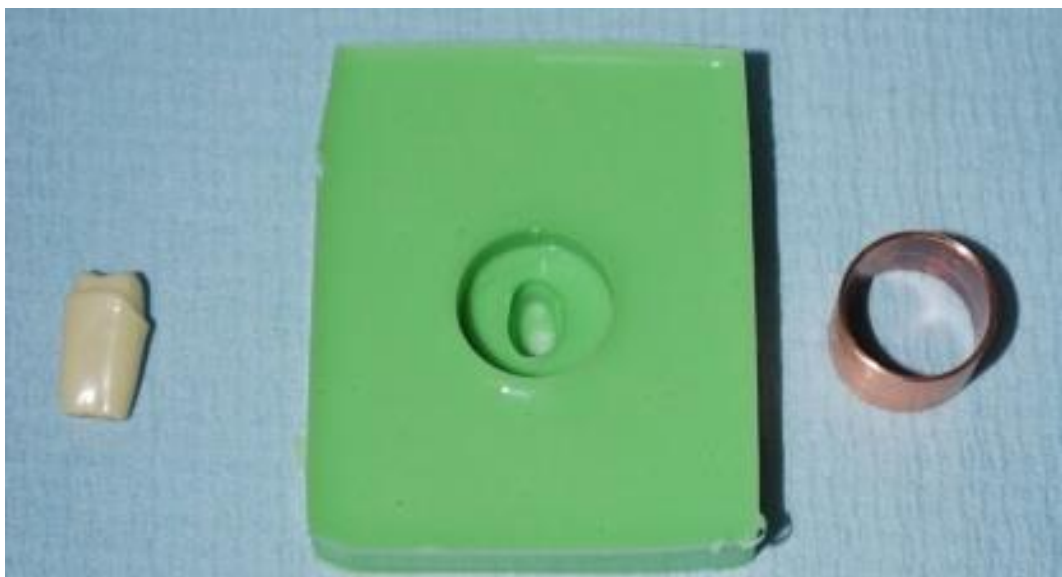
Figure 8-5: the mould of the ideal alignment of the samples
