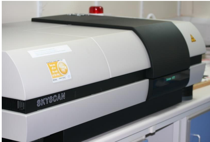
Figure 5-3: Sky scan micro-CT scanner
