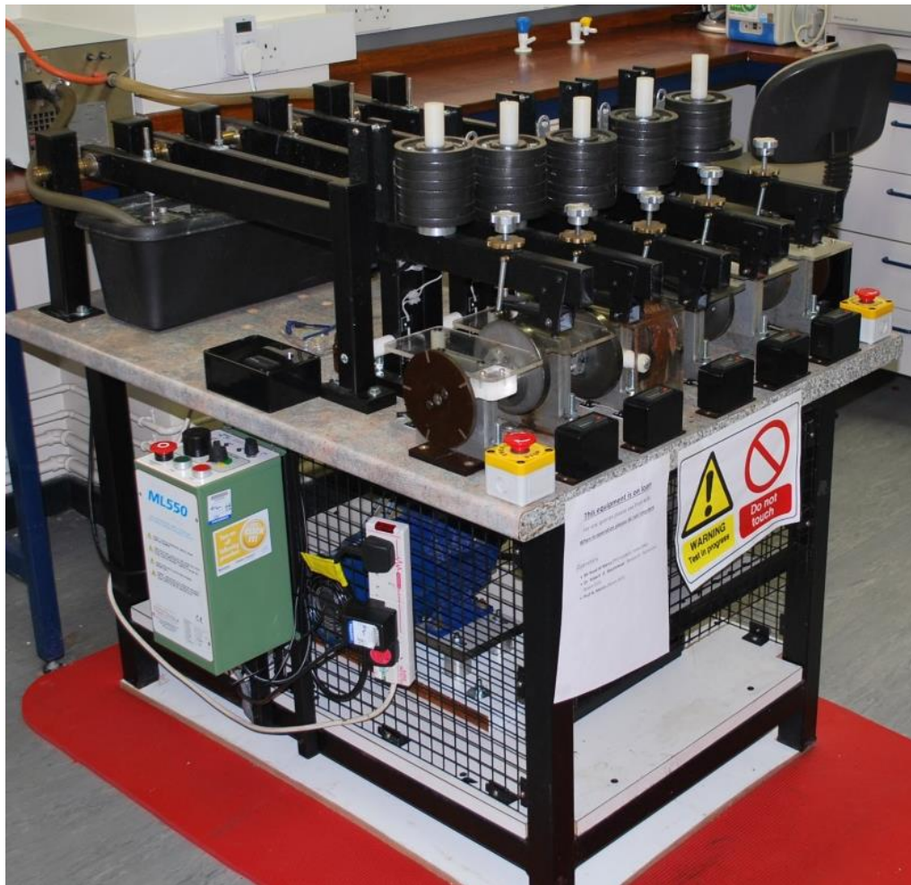
Figure 8-9: Fatigue machine tester
