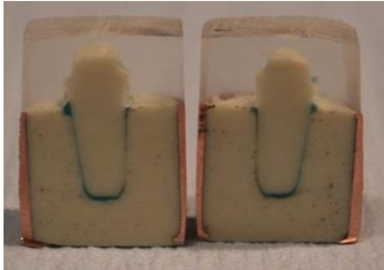
Figure 8-7: PDL simulation (tooth crown embedded in acrylic for this specimen to facilitate sectioning that enables visualisation of the tooth and PDL in cross-section)
