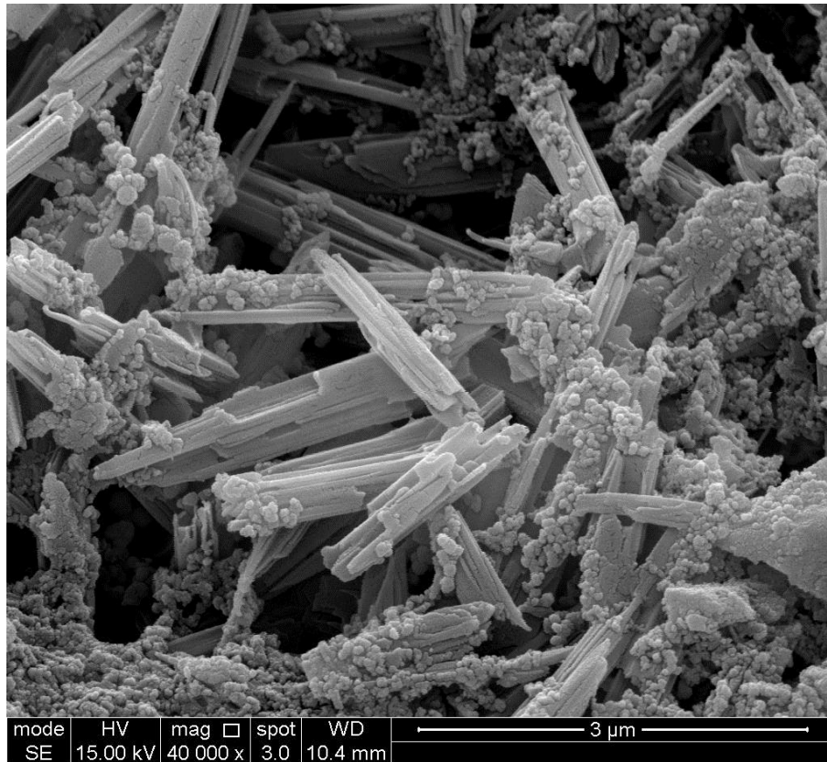
Figure 6-33: SEM of etched e.max ® pressed at 40000x
