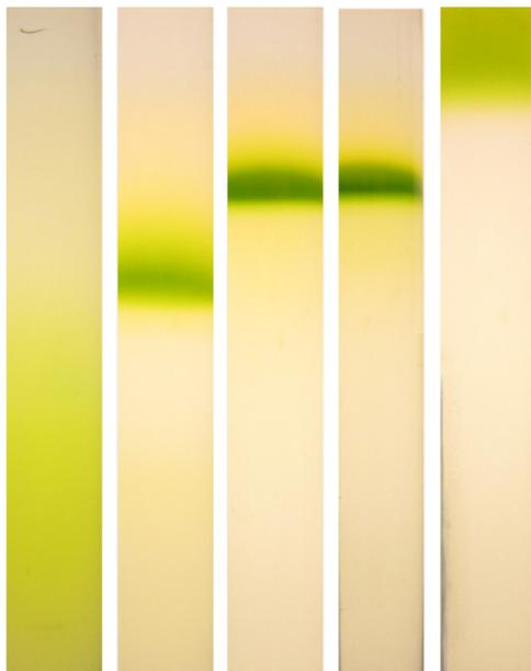
**Figure 3.17. Secondary sucrose gradients from  $\beta$ -DDM trial.** The concentrations of  $\beta$ -DDM in the gradients from left to right were; 0.000 % (control gradient), 0.001 %, 0.005 %, 0.01 % and 0.05 %. The green fraction travels less distance through the gradient as the detergent concentration increases indicating the size of the membrane fragments is decreasing
