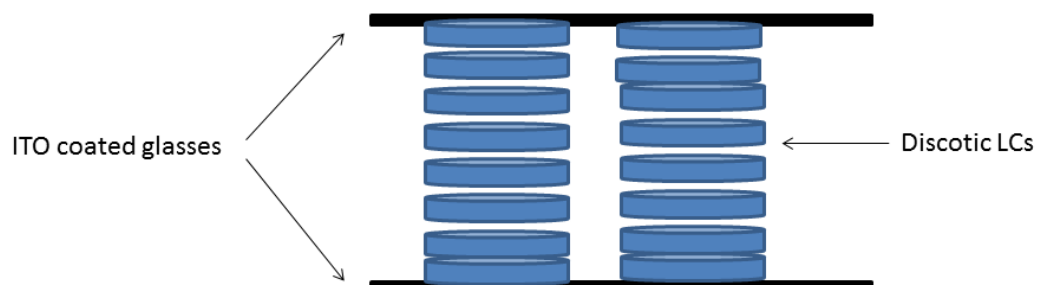
Figure 4.76 Schematic representation of homeotropic alignment.
