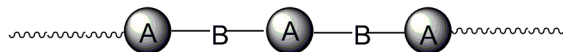
Figure 1.2 Schematic representation of typical structure of rod-like LCs; A represents ring structure, B represents linking group.
