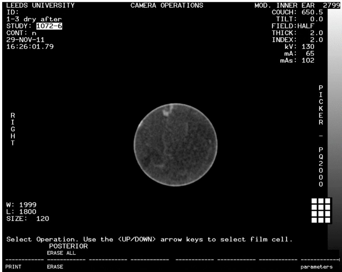
**Figure 3.5** 2mm thick cross section of a Cayton Bay rock core as seen in the PICKER PQ 2000 medical CT scanner.
