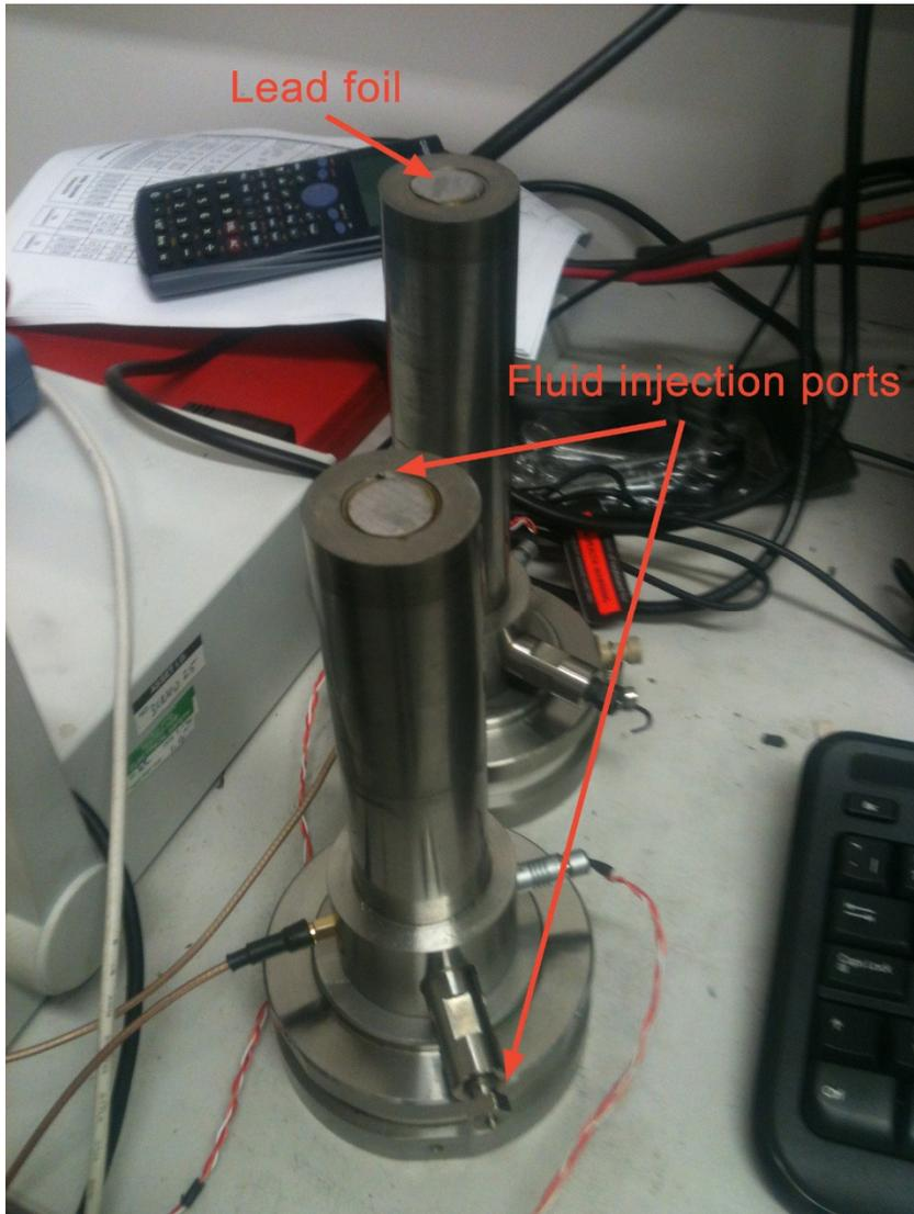
**Figure 5.2** Steel platens placed on both sides of the sample inside the heater and used to generate sonic waves and to inject fluids.
