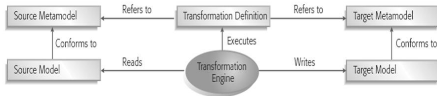
Figure 2.10: Basic concepts of model transformation [CH06]
