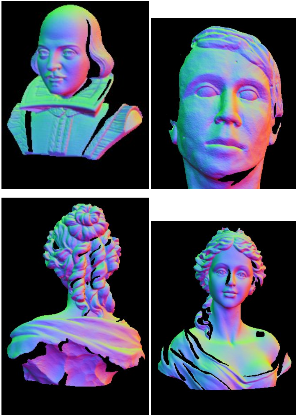
Figure 4.11: The ground truth normal maps for the four input images, as calculated using a head scanner. For calculating the error only areas where data is present are used, the black masked out regions are either background or where the scanner failed due to occlusion.
