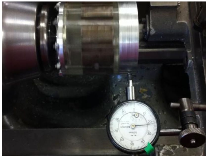
Fig. 2.37. Measurement of rotor eccentricity using a comparator and lathe.
