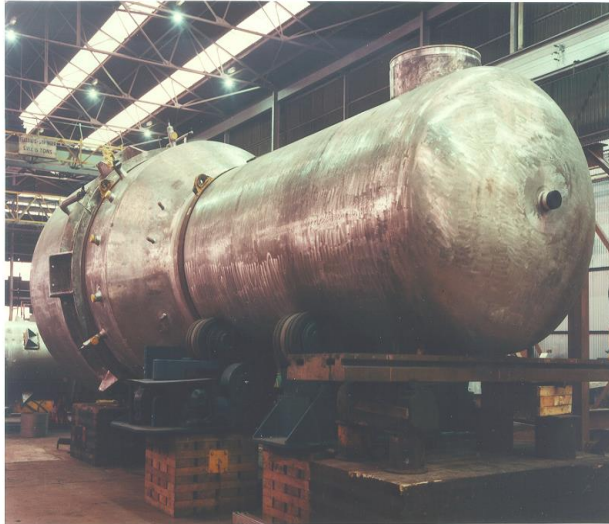
Figure 2.3-2 Image representing evaporator C prior to installation. The top of the vessel is in the foreground (NNL, 2008c).
