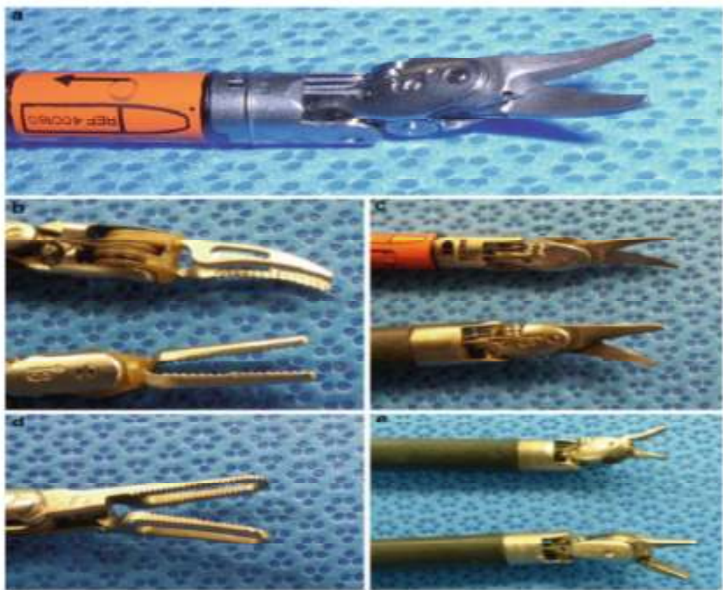
Figure 2.6 Figures of articular grasping jaws for the robotic surgery (Diodato Jr et al., 2004).
