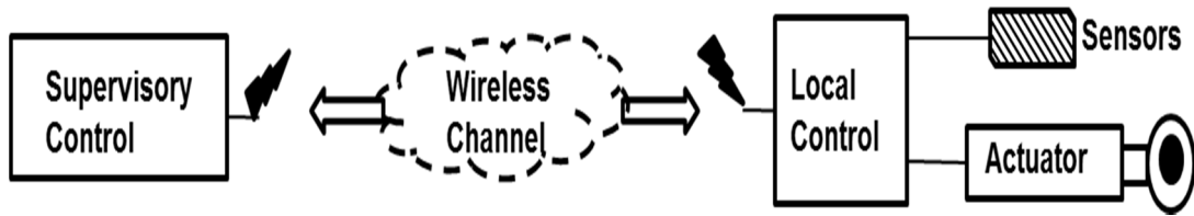
Figure 4.2: Supervisory wireless real-time closed-loop control system
