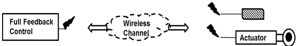
Figure 4.3: Full feedback wireless real-time control system
