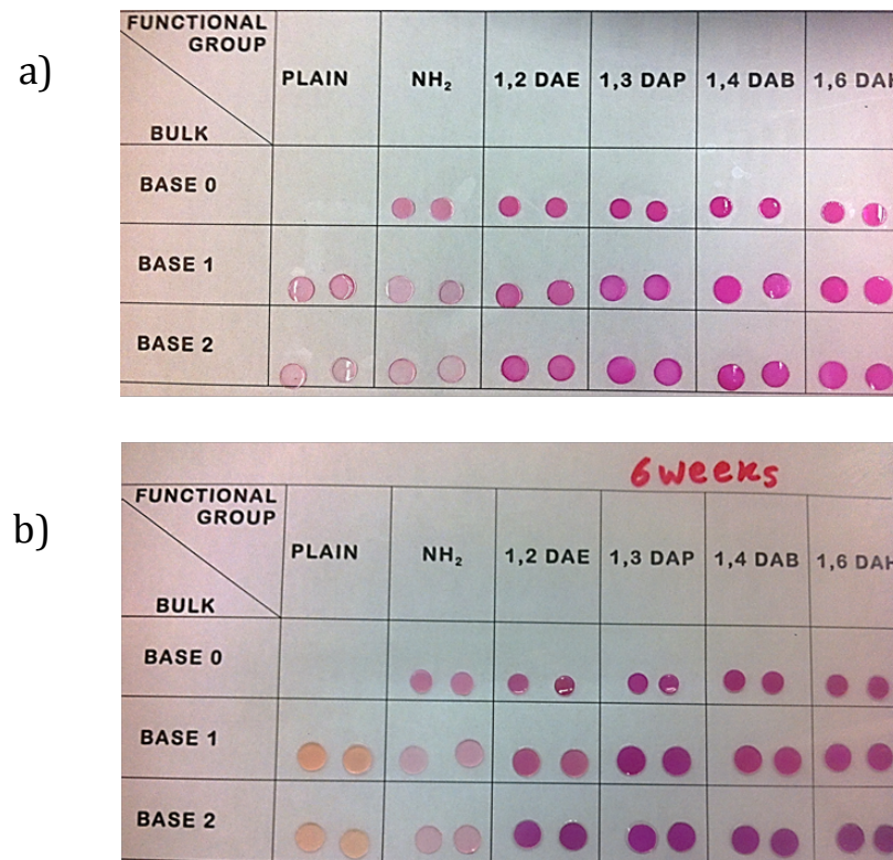
FIGURE 4.19: Photographs of hydrogel discs immersed in media containing phenol red for 24 hrs then washed in PBS (a) and the change in pH of media over 6 week saturation at 37°C (b).
