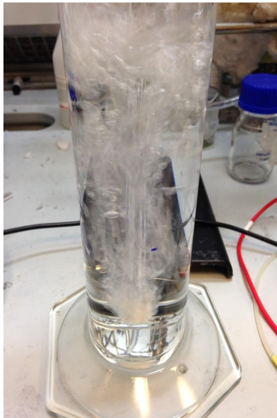
Figure 0-7 Heterogeneous flow regime at higher flow rates ( 2\text{-}5 \text{ l min}^{-1} ) in the current study
