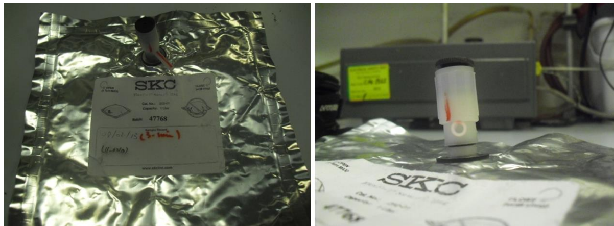
Figure 5-15 SKC-H 2 storage bad and inlet orifice
