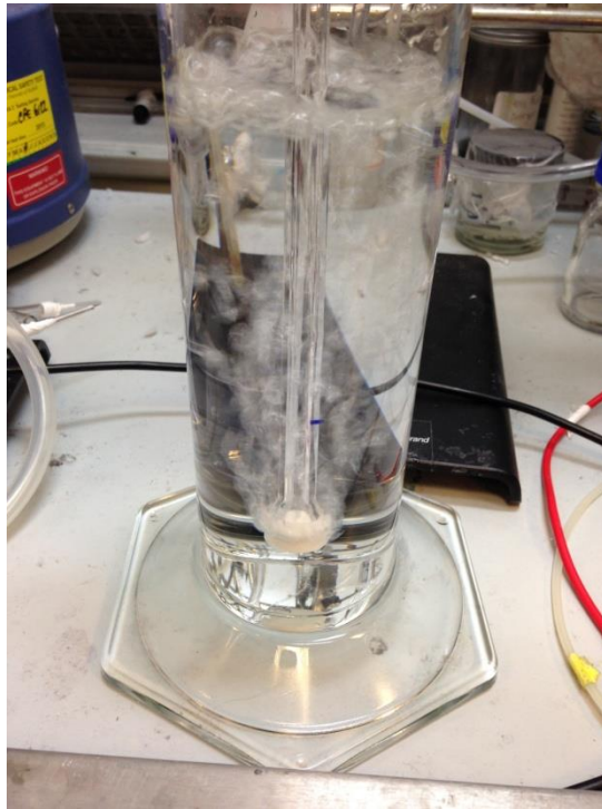
Figure 0-6 Bubble flow regime at relatively lower flow rates ( 1 \text{ l min}^{-1} ) in the current study
