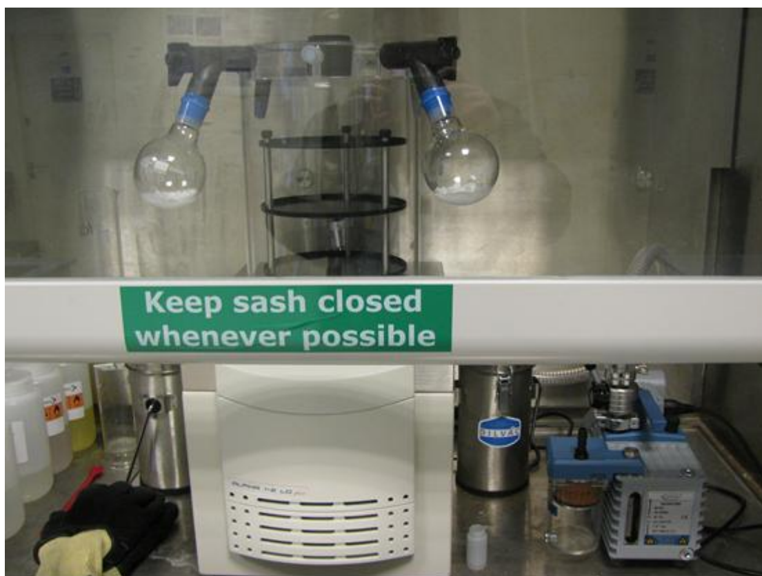
Figure 3.3 – Photo of Christ Alpha 1-2LD plus freeze dryer
