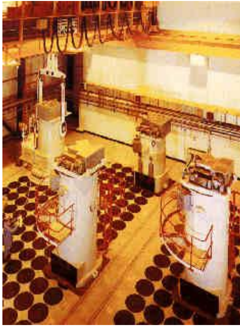
Figure 2.12 – The interim storage facility for vitrified HLW at Sellafield (World Nuclear Association, 2008b)
