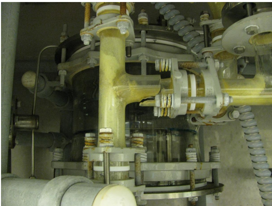
Figure 4.6 – Photo showing fracture of the glassware during testing of the small scale calciner
