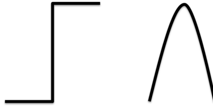
Figure 7.1: Time derivative relationship btw. DC and RF. By advancing to spatially extended sources an extra time derivative is introduced in the displacement. This may lead to misinterpretation of magma ascent (step function) as initially ascending, but then stagnating (pulse) magma.
