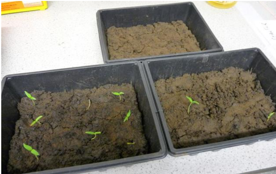
Plate 6.2: Test trays containing contaminated soil, the seedlings are struggling and less robust unlike the controls in Plate 6.1. The tray to the left contains 5% oil w/w, the tray to the right contains 7.5% oil w/w and the tray behind contains 10% oil w/w
