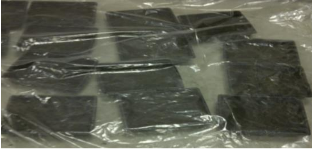
Plate 3.3: Day 1 showing the trays covered with plastic sheet to reduce any interference with germination. The plastic sheet was removed after 70% germination was observed in the control trays
