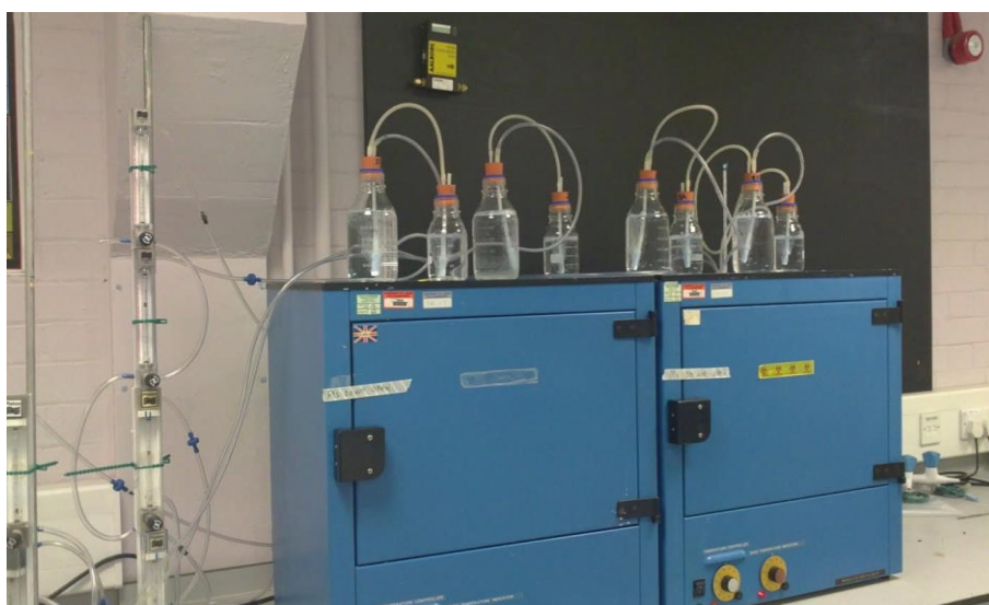
Plate 3.1: Laboratory set-up of DR4 apparatus housing more than one reactor
